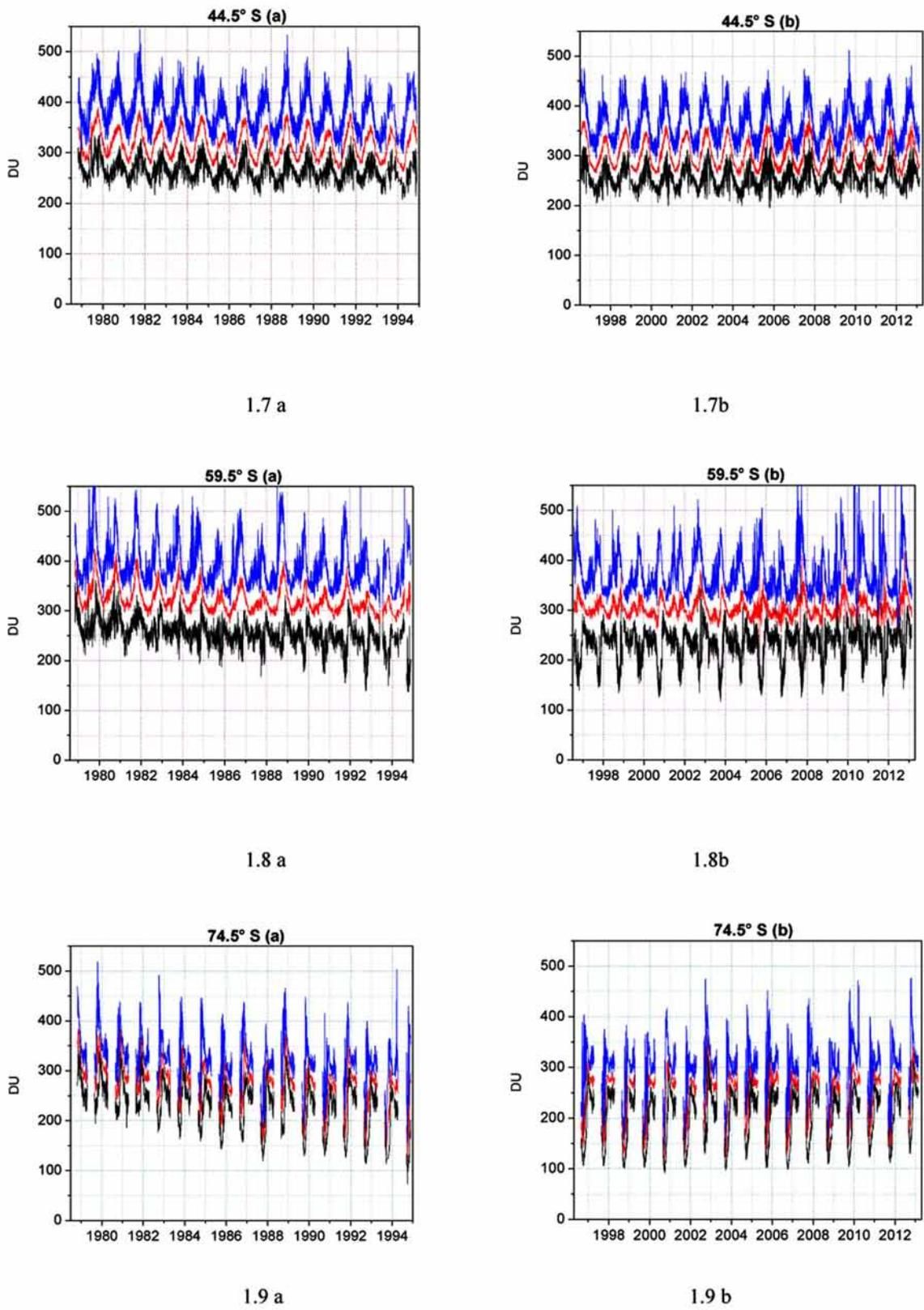
**Fig. (1).** Latitudinal daily behavior of the largest (blue) mean (red) and smallest (black) measurements of the TCO at nine selected 1°-latitude bands.
