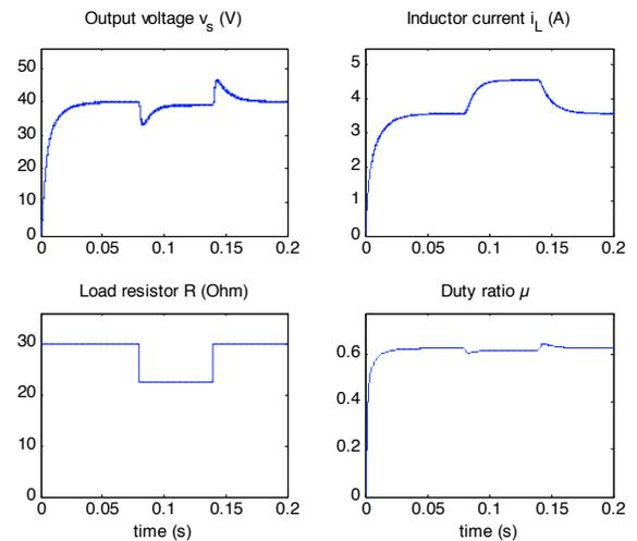
Fig. (7). Controller behavior for load resistance change.
