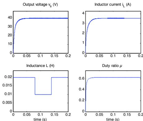
Fig. (5). Controller behavior for inductance change.
