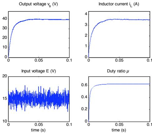
Fig. (4). Controller behavior for input voltage change.
