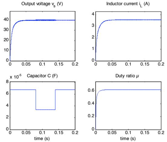
Fig. (6). Controller behavior for capacitor change.
