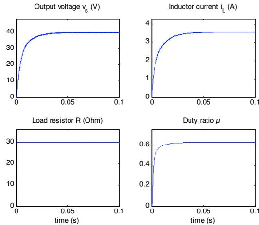
Fig. (3). Controller behavior in presence of step reference  $V_d = 40V$  and invariant parameters
