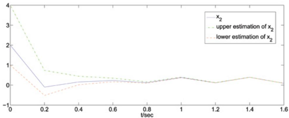
Fig. (3). Evolution of the real state  $x_2(k)$  and the estimations  $\hat{x}_2^+(k)$ ,  $\hat{x}_2^-(k)$
