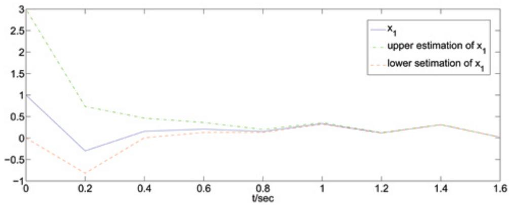
Fig. (2). Evolution of the real state  $x_1(k)$  and the estimations  $\hat{x}_1^+(k)$ ,  $\hat{x}_1^-(k)$
