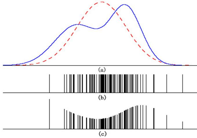
**Fig. (3).** The importance weight description: the dotted line in (a) represents suggestion distribution and the solid line represents actual distribution; (b) shows the sample from suggestion distribution while (c) shows the distribution of the sample after modification.
