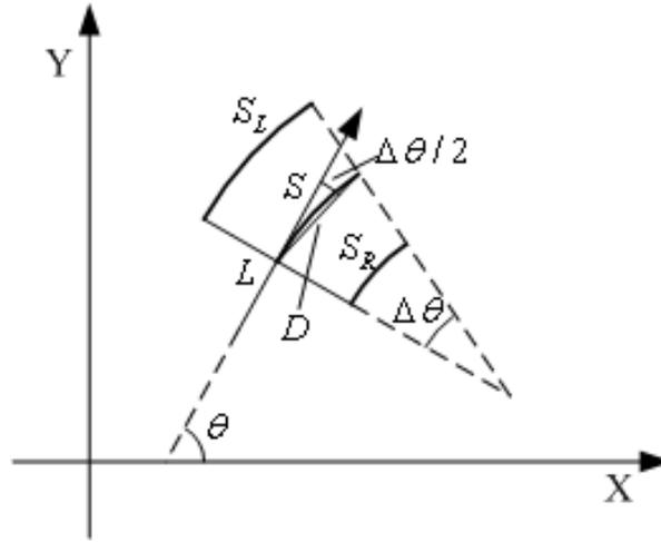
Fig. (5). The moving model of robot wheels.
