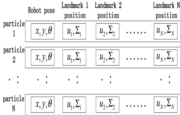
Fig. (2). The filter structure of FastSLAM, a total of  $M$  particles in filter and each particle owns distinct  $N$  EKF filters.
