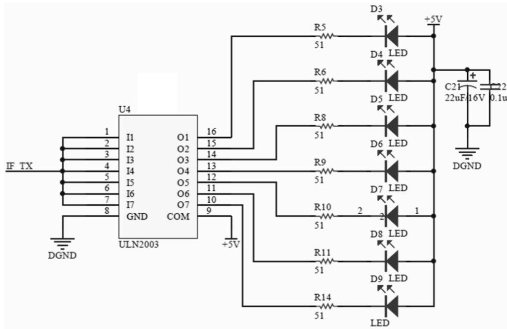
Fig. (10). Circuit diagram of infrared emitter.
