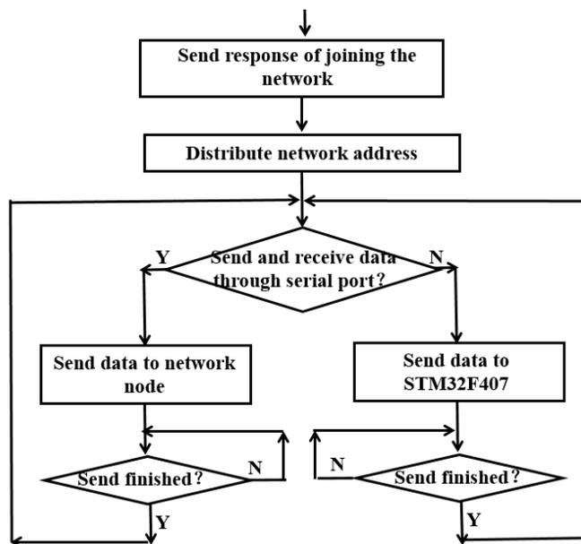
Fig. (13). Flowchart of ZigBee coordinator program.
