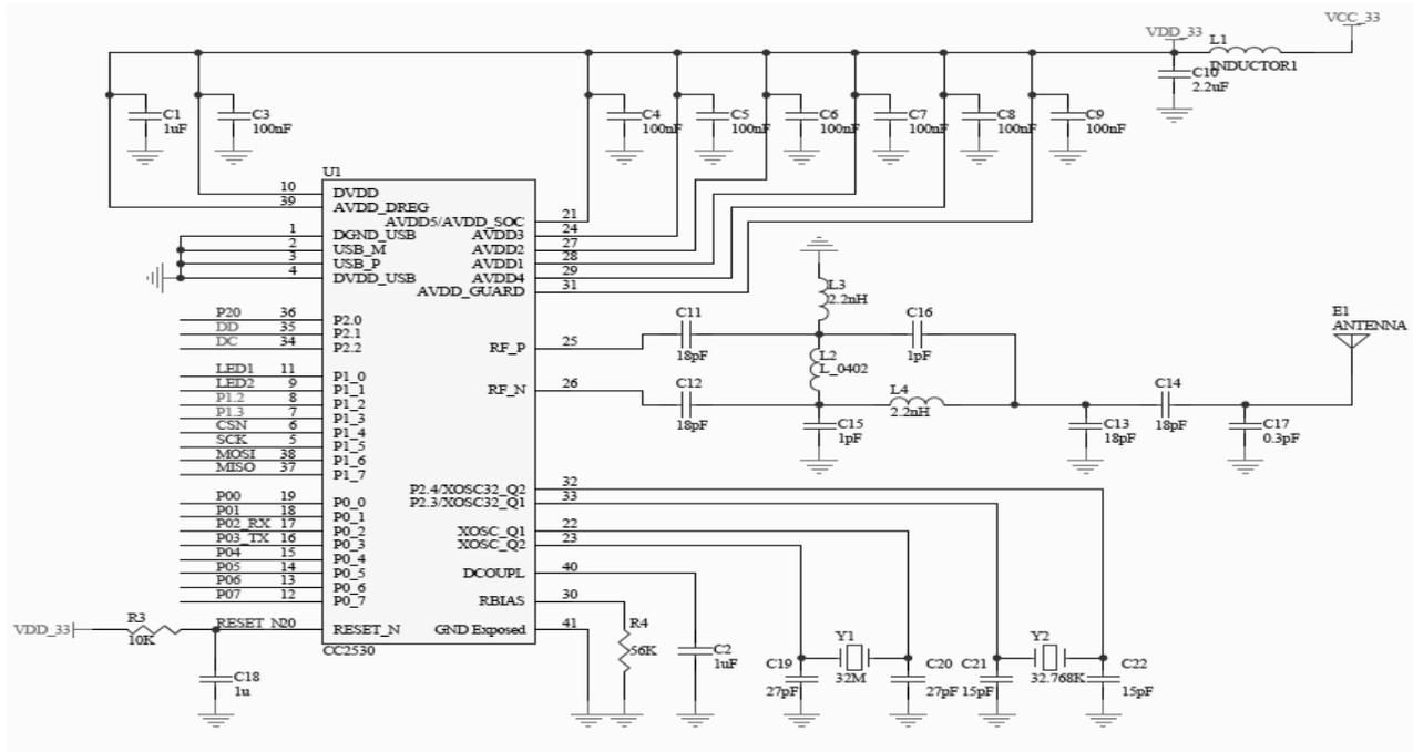
Fig. (3). CC2530 typical circuit.
