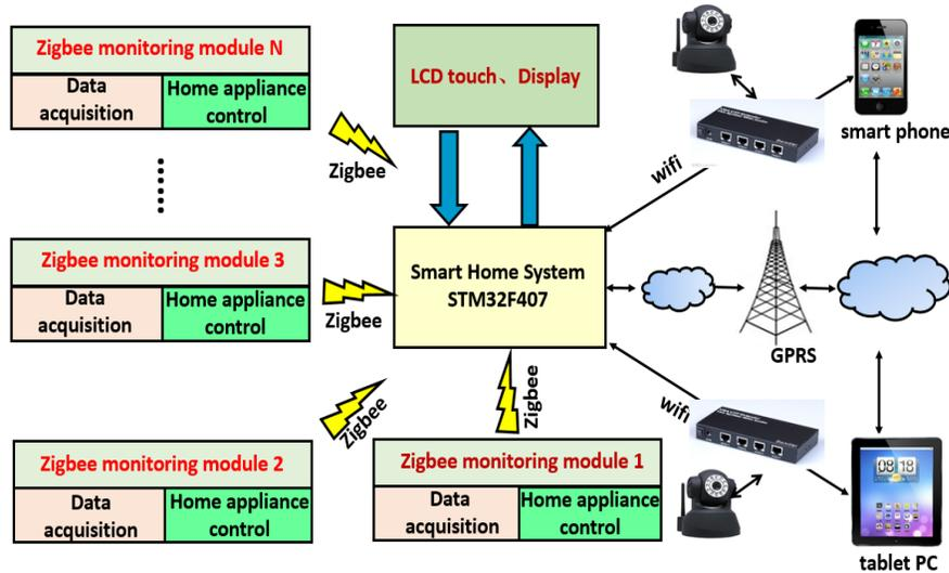
Fig. (1). Overall structure of the smart home system.
