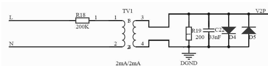
Fig. (6). Circuit diagram of voltage acquisition in the power network.
