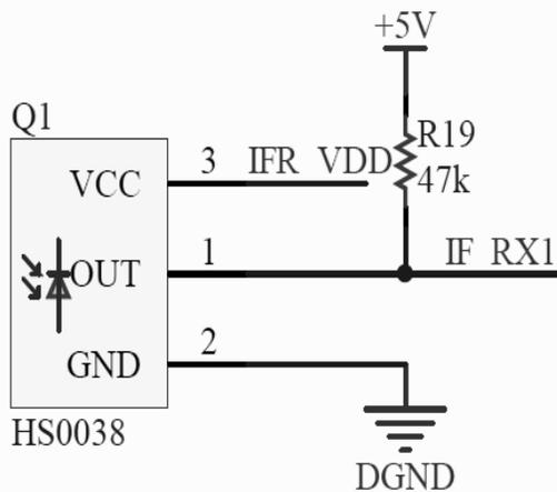
Fig. (9). Circuit diagram of infrared receiver.
