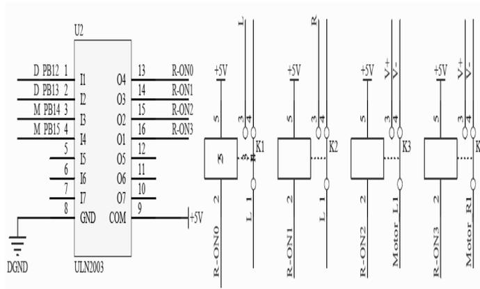
Fig. (11). Circuit diagram of electric curtains.
