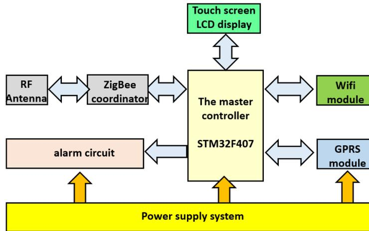
Fig. (2). Structure of the master controller.
