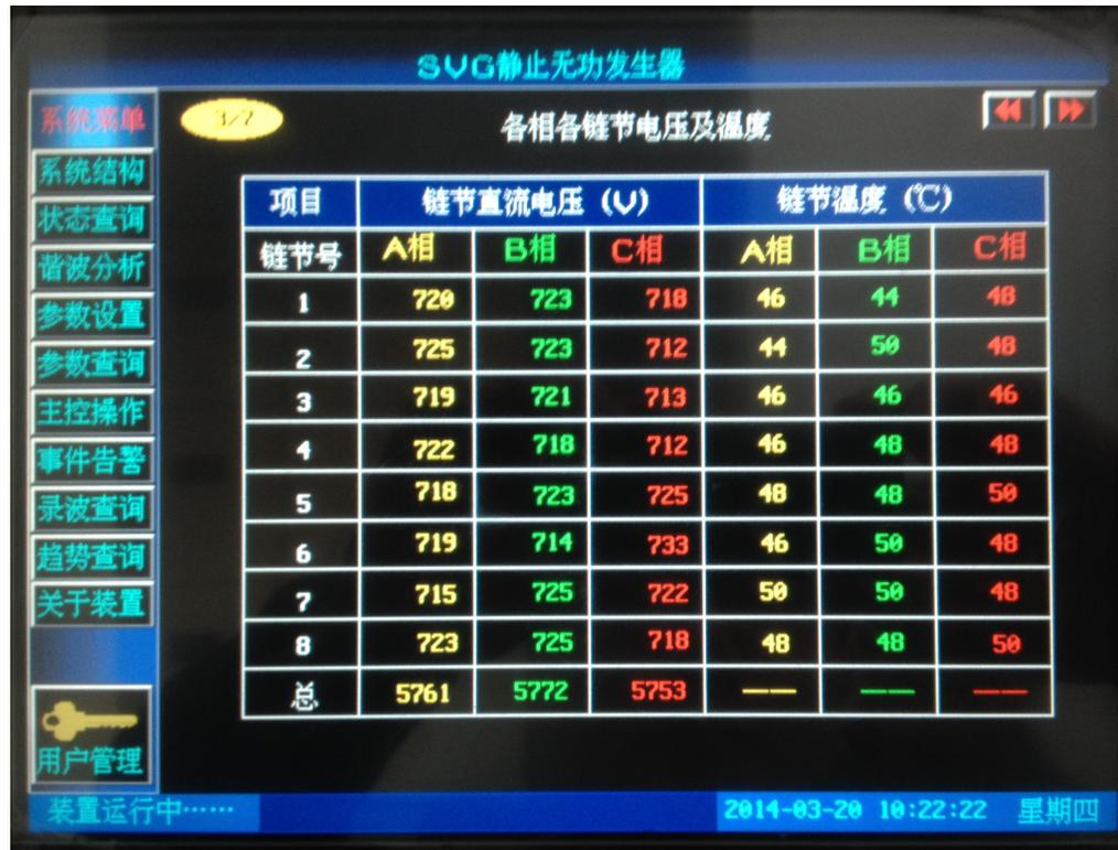
Fig. (8). DC capacitor voltages.
