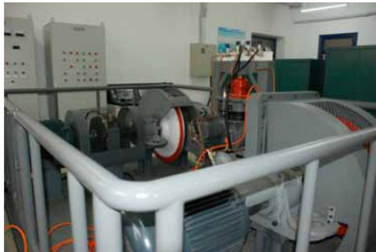
Fig. (6). Data acquisition and processing test bed of the brake controller.
