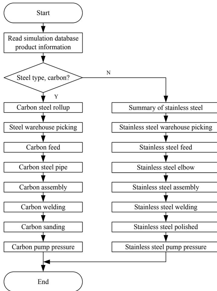
**Fig. (1).** Simulation flow chart of pipe processing plant.
