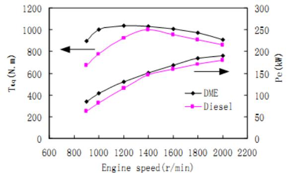
**Fig. (1).** Comparison of torque and power of DME engine and diesel engine at full load.
