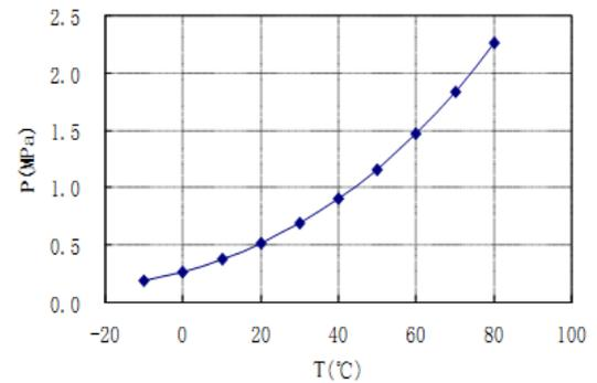
**Fig. (5).** Effect of temperature on vapor pressure of DM.
