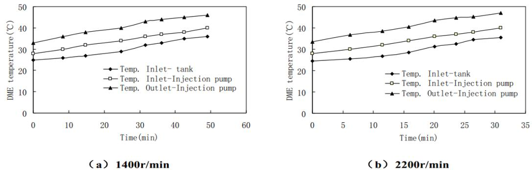
**Fig. (2).** Variation of DME temperature with time (injection advance angle 8°CA BTDC, P8500 Pump, 12 mm Piston, 6 × 0.43 mm Nozzle).
