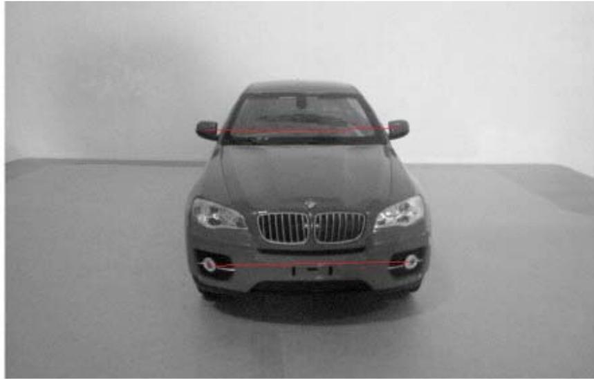
Fig. (7). Detected symmetric pairs of feature points in left image.
