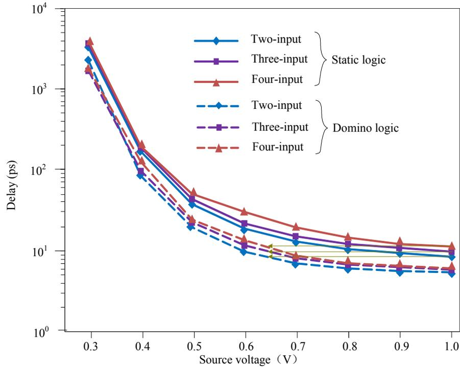
Fig. (2). Propagation delay of 32nm NAND/AND gates based on static and Domino FinFET logic, where the operation frequency is chosen by the minimum value of maximum operation frequencies of the static and Domino logic gates.
