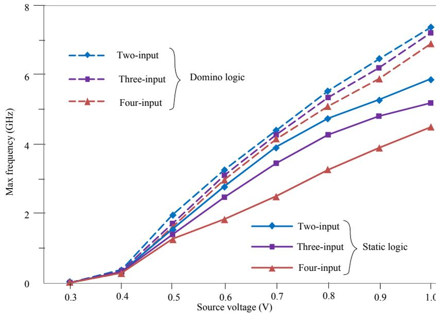
Fig. (5). Maximum operation frequency of 32nm NAND/AND gates based on static and Domino FinFET logic.
