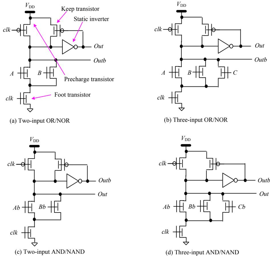
Fig. (1). Two-input and three-input OR/NOR and AND/NAND FinFET gates.
