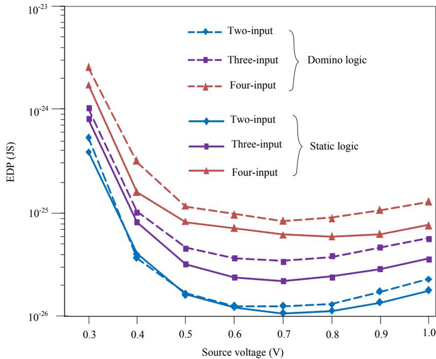
**Fig. (4).** EDP of 32nm NAND/AND gates based on static and Domino FinFET logic.
