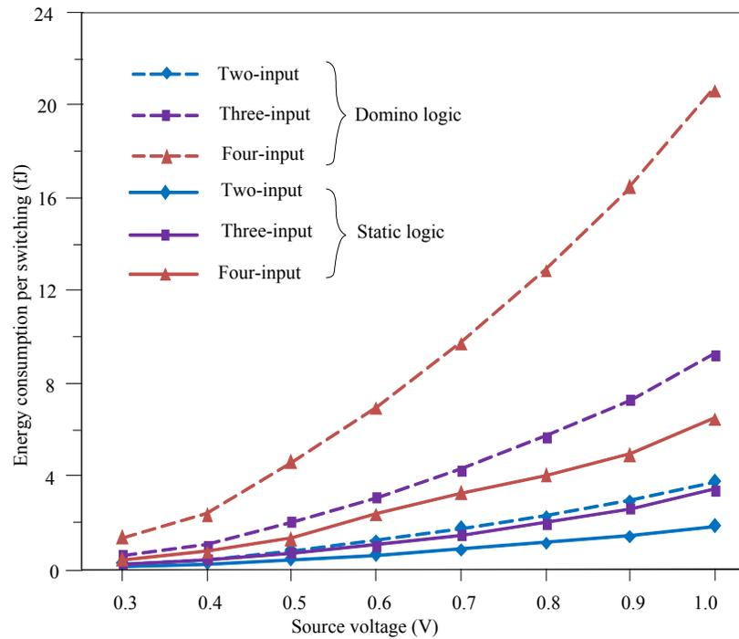
**Fig. (3).** Energy consumption per switching of 32nm NAND/AND gates based on static and Domino FinFET logic, where the operation frequency is chosen by the minimum value of maximum operation frequencies of the static and Domino logic gates.
