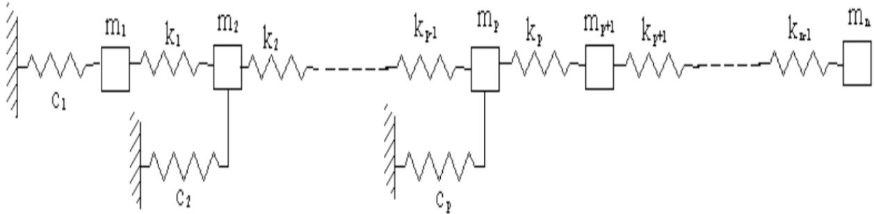
Fig. (1). A grounding spring-mass system.
