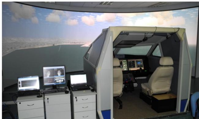
Fig. (4). The flight simulator and monitoring system.
