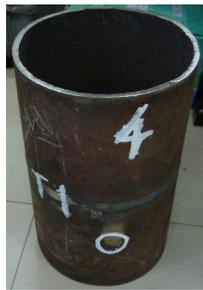
Fig. (1). Butt welded tubular specimen.
