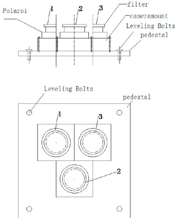
Fig. (3). Schematic diagram of detection device.
