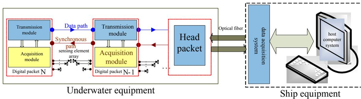
Fig. (1). Towed Linear Sonar System Structure.
