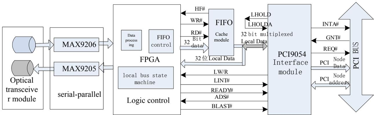
Fig. (3). Hardware Structure of Data Recording System.
