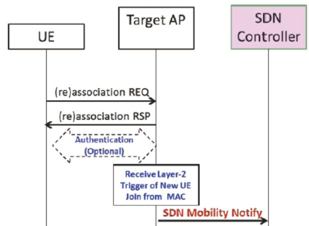
Fig. (5). The Information trigger process of the SDN Mobility Management Notify-the later trigger after the ending of the Layer-2 procedure.
