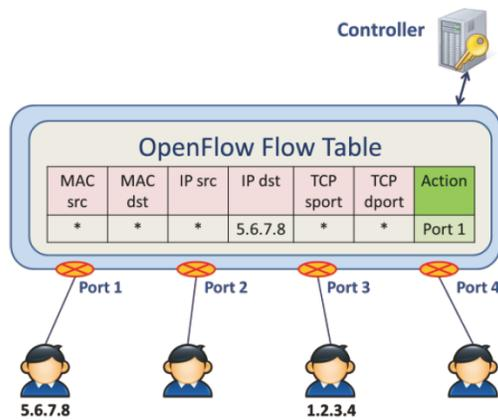
Fig. (2). The framework of the SDN.
