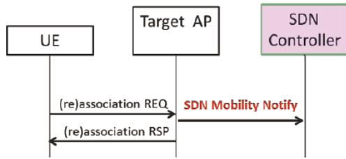
**Fig. (6).** The Information trigger process of the SDN Mobility Management Notify-the trigger after the information of the first Layer-2 is delivered to the AP.
