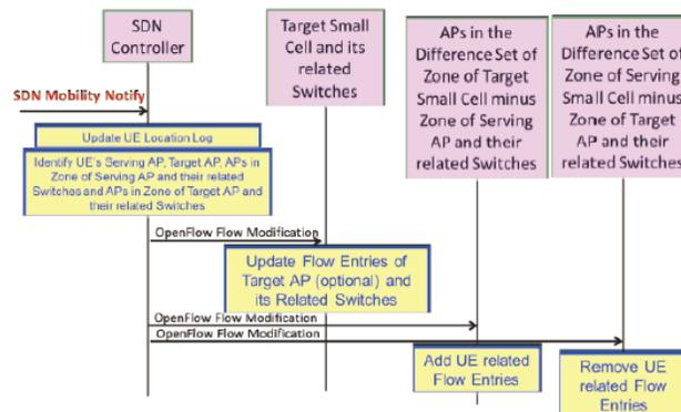
**Fig. (7).** The information processing procedure in the SDN Mobility Management Notify.
