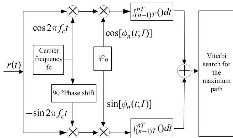
Fig. (6). The diagram of ML-Viterbi demodulation.
