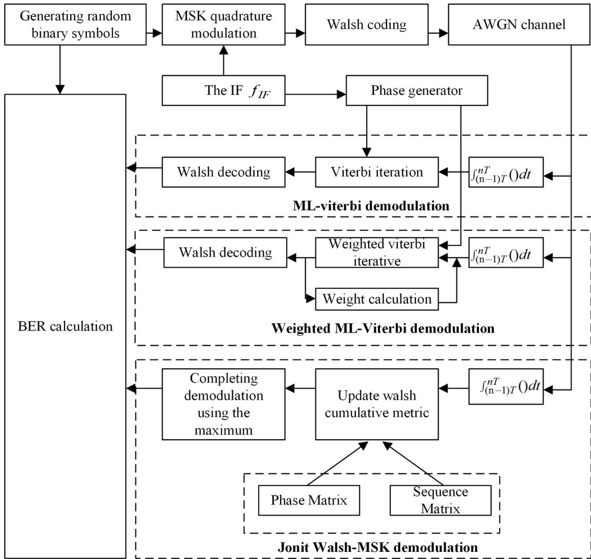
Fig. (12). The flow of joint demodulation and despreading algorithm.
