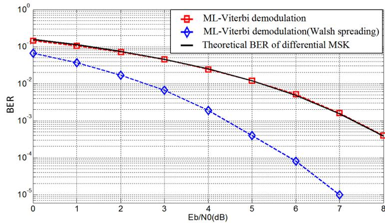
Fig. (13). BER curves of basic ML-Viterbi demodulation algorithm.
