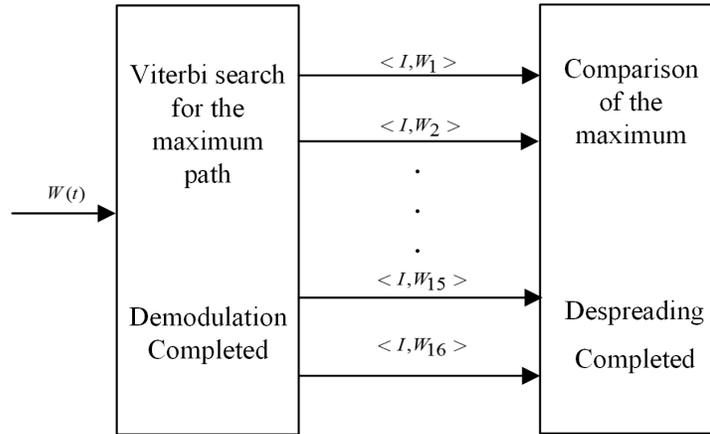
Fig. (8). The block diagram of Walsh despreading.
