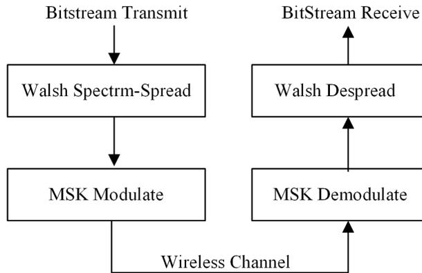
Fig. (2). MOD-5 signal process flow.
