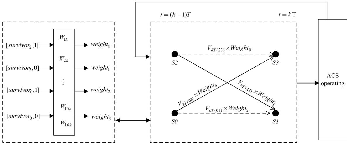
Fig. (9). Calculation of the additional increment in Weight-ML-Viterbi algorithm.
