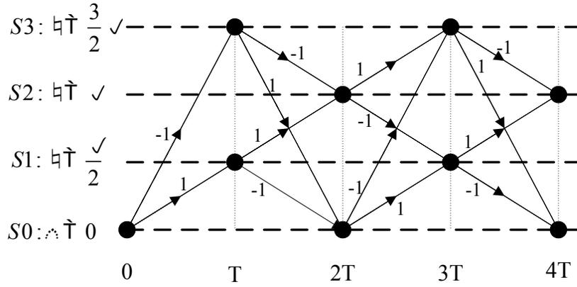
Fig. (7). Phase change trellis of MSK signal.
