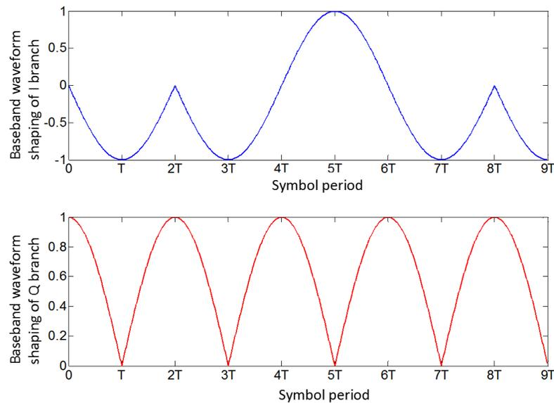
Fig. (4). Example of MSK modulation IQ waveform.
