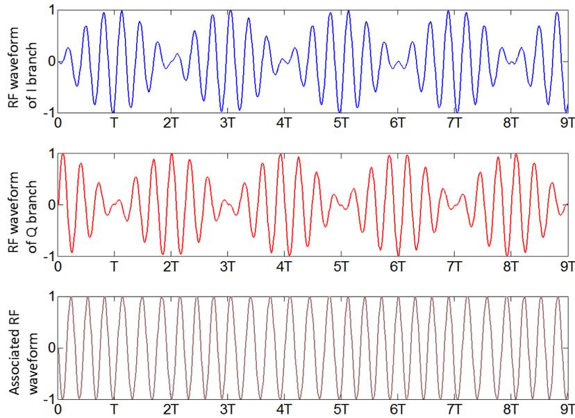
Fig. (5). MSK RF waveform.
