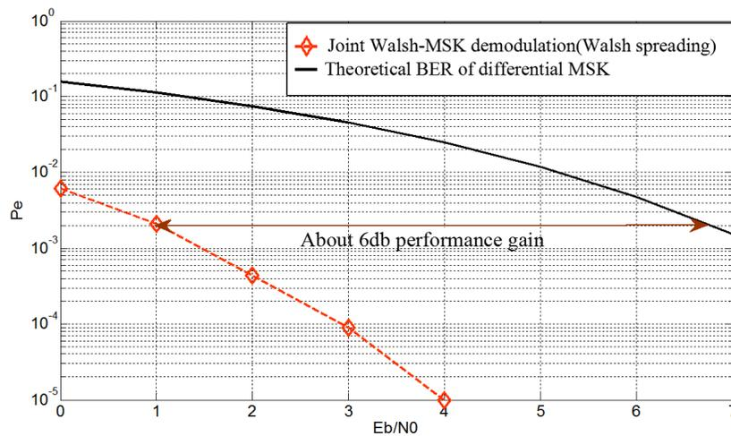
Fig. (15). BER curves of joint demodulation and despreading algorithm.
