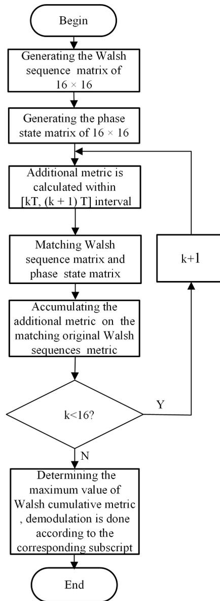
**Fig. (11).** Flow of joint demodulation and despreading algorithm.
