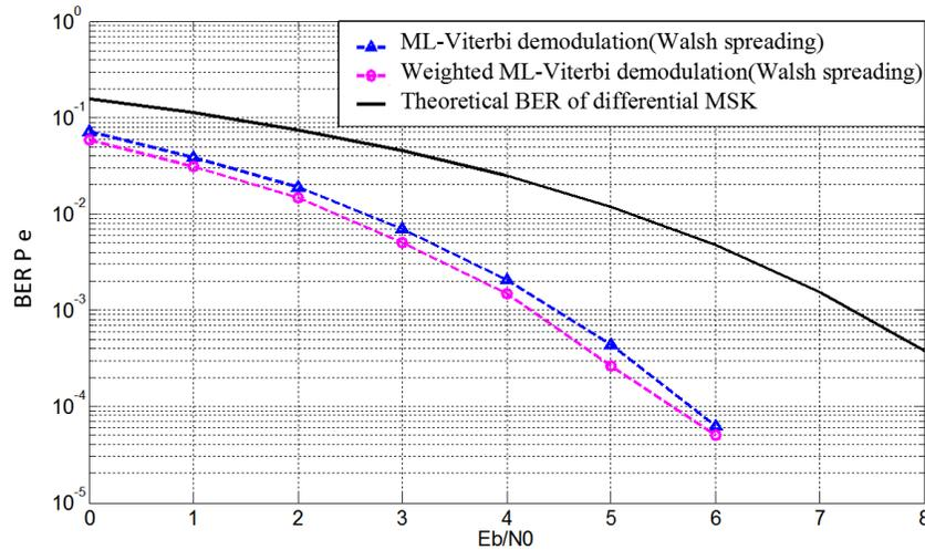
Fig. (14). BER curves of weighted ML-Viterbi demodulation algorithm.
