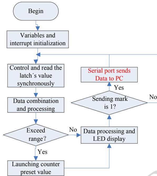
Fig. (8). The flow diagram of data processing.
