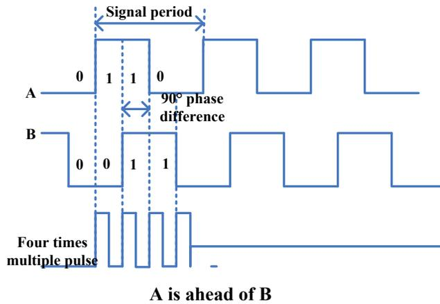
Fig. (5). The principle of four times subdivision.
