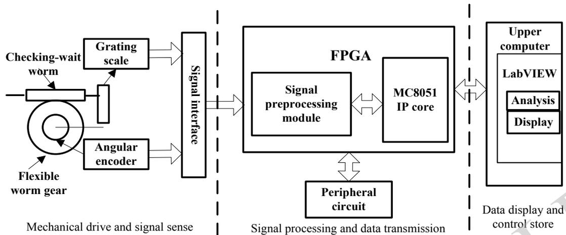
Fig. (1). The whole system block diagram.
