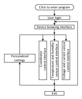
Fig. (3). Software flowchart of the mobile client.
