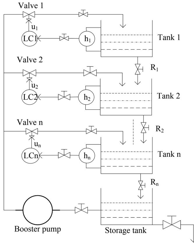
Fig. (1). Schematic diagram of multi-tank system.
