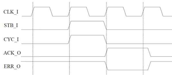
**Fig. (5).** Wishbone handshaking protocol with master.
