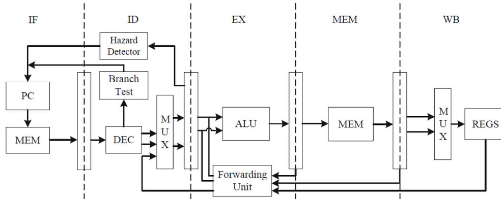
Fig. (3). Pipelined datapath.
