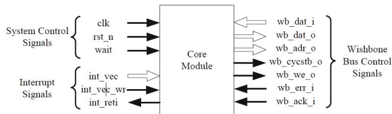
Fig. (2). Top interface of core module.
