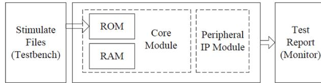
Fig. (10). Verification platform of system integration.
