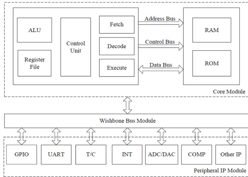
Fig. (1). System structure of YL8MCU.
