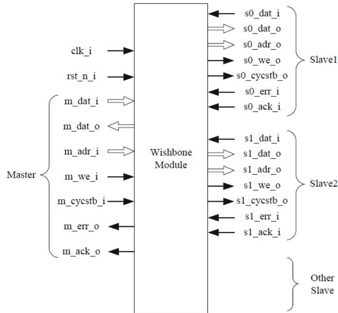
Fig. (6). Top interface of Wishbone bus module.
