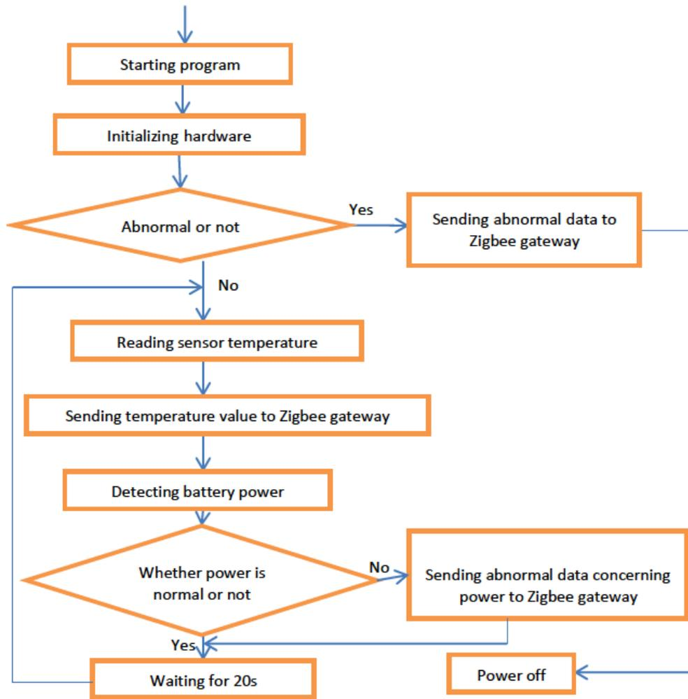
Fig. (2). Temperature detecting algorithm flow chart.
