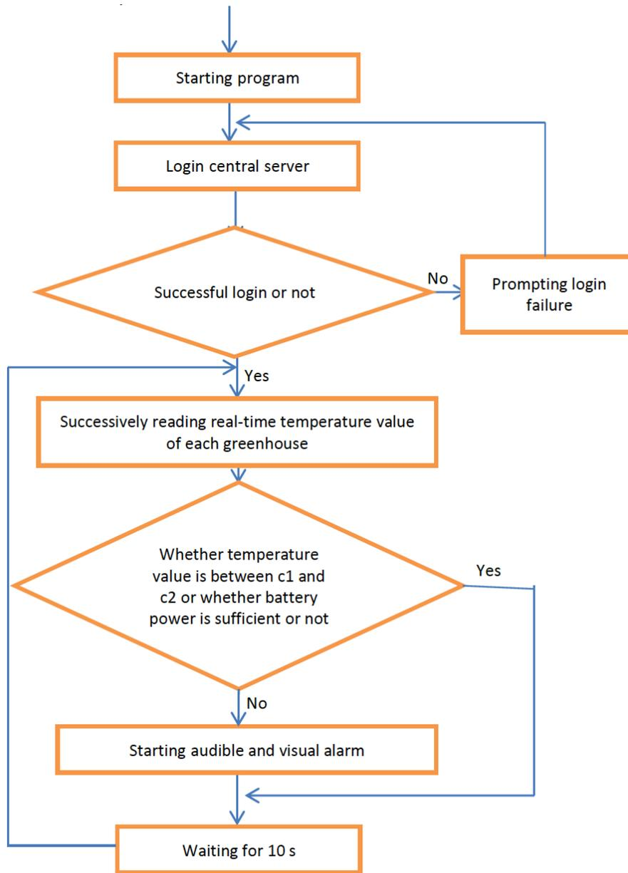
Fig. (3). Temperature warning algorithm flow chart.
