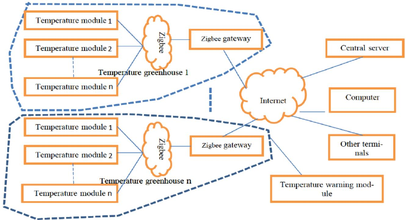
Fig. (1). Overall structure of the system.
