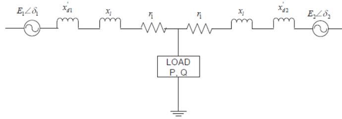
Fig. (1). Block diagram of the two-parallel model.
