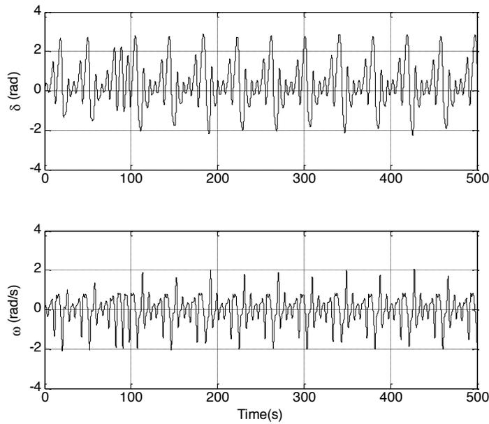
Fig. (3). Timing diagram of power angle  $\delta$  and relative power angle velocity  $\omega$ .
