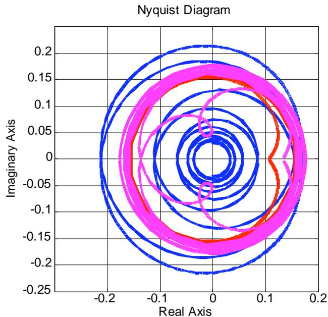
**Fig. (3).** Nyquist diagram for the Example 1 systems. For  $h = 1$ ,  $\bar{p}(j\omega)$ : solid blue line,  $\bar{p}_1(j\omega)$ : dashed red line,  $\bar{p}_2(j\omega)$ : dotted magenta line.
