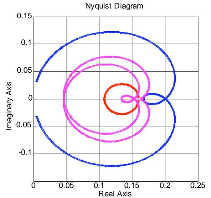
**Fig. (2).** Nyquist diagram for the Example 1 systems.  $p(j\omega)$ : solid blue line,  $p_1(j\omega)$ : dashed red line,  $p_2(j\omega)$ : dotted magenta line.
