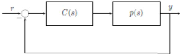
**Fig. (1).** Unity feedback.  $r$ : reference signal,  $y$ : system output,  $C(s)$ : controller,  $\bar{p}(s)$ : system.
