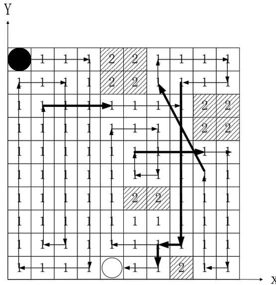
**Fig. (9).** The path of ISS in the environment with multiple regular obstacles.
