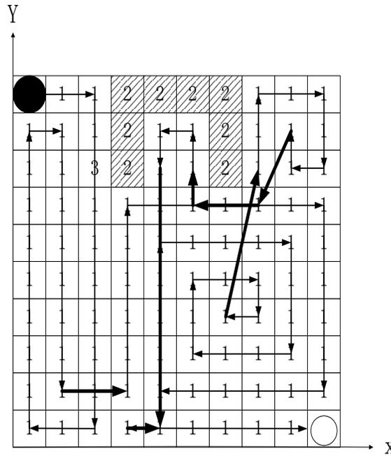
Fig. (7). The path of ISS in the environment with irregular obstacles.
