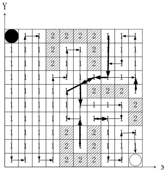
**Fig. (10).** the path of UAPP algorithm in the environment with multiple irregular obstacles.
