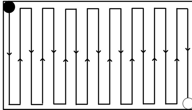
Fig. (1). The map of U-turn algorithm. It uses “●” to indicate the starting point of cleaning robot, and uses “○” to indicate the ending point position of cleaning robot. The back of the figure have the same representation.
