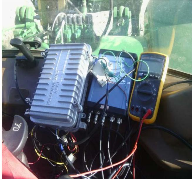
**Fig. (12).** The controller used in the tractor automatic navigation.
