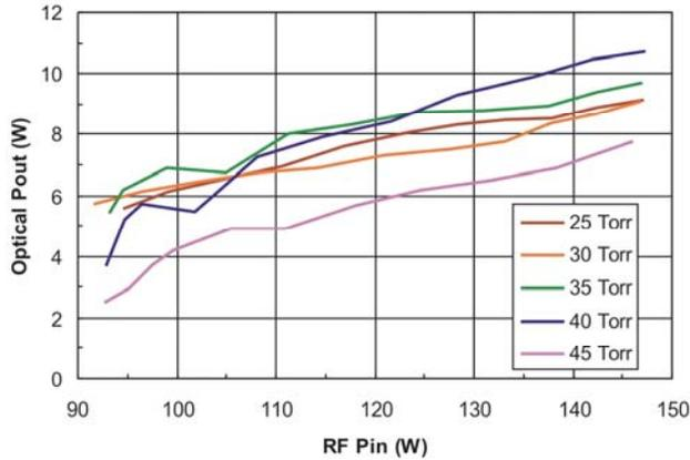
**Fig. (6).** Laser output power extraction versus the RF input power from the two stage circuit and using different final pressure in the laser amplifying media.
