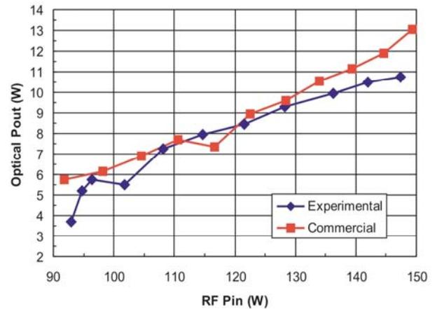
**Fig. (8).** Laser performance using both, a commercial and our experimental RF power supply.
