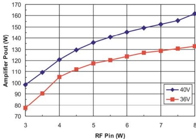
Fig. (3). Amplifier output power in terms of the oscillator RF signal taken as input for the amplifier stage.
