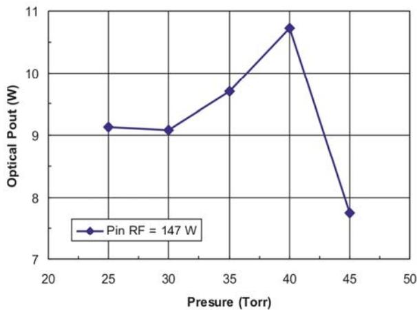
**Fig. (7).** Optical power variations for different gas pressures in the laser amplifying medium.
