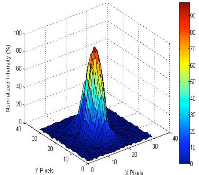
**Fig. (9).** Experimental laser beam profile recorded as mode TEM<sub>00</sub>.
