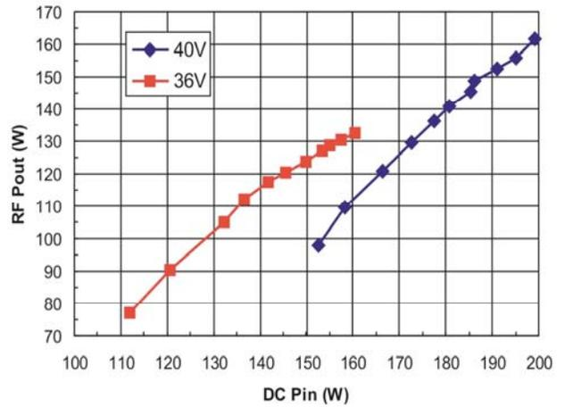
Fig. (4). Output power versus DC Input Power of the power supply.
