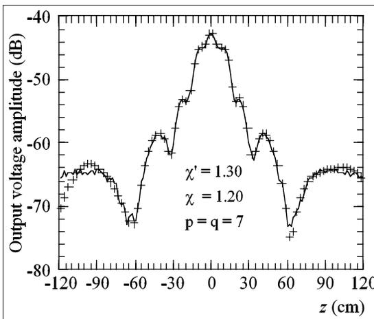
Fig. (4). Amplitude of the probe voltage on the generatrix at  $\varphi = 30^\circ$ . Solid line: measured. Crosses: interpolated.
