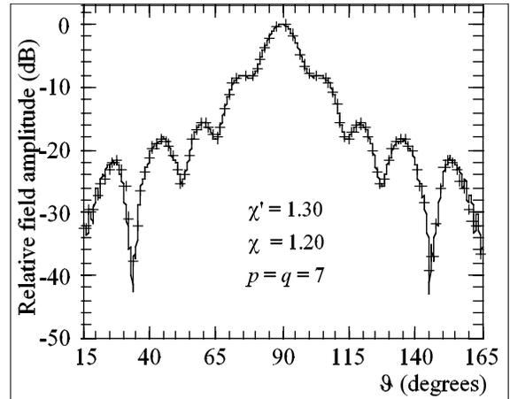
Fig. (6). E-plane pattern. Solid line: reference. Crosses: reconstructed from NF data acquired *via* helicoidal scanning.
