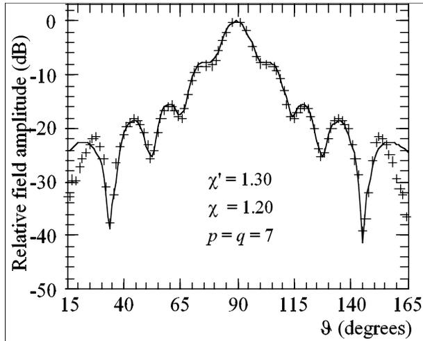
Fig. (8). E-plane pattern. Solid line: direct FF measurements. Crosses: reconstructed from NF data acquired via helicoidal scanning.
