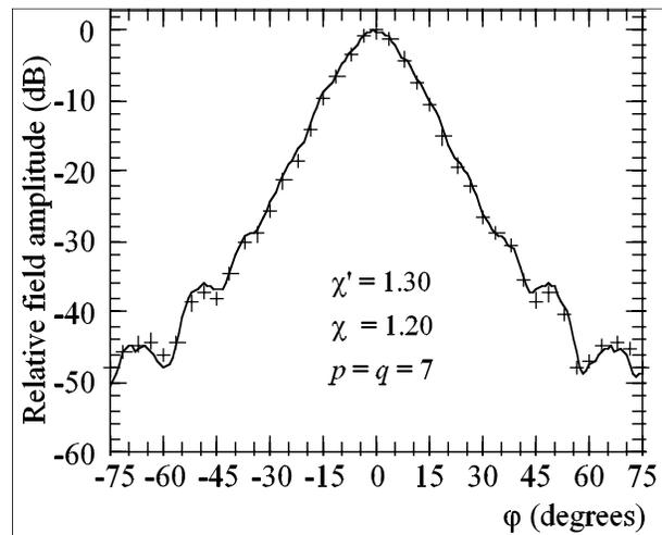
Fig. (9). H-plane pattern. Solid line: direct FF measurements. Crosses: reconstructed from NF data acquired via helicoidal scanning.
