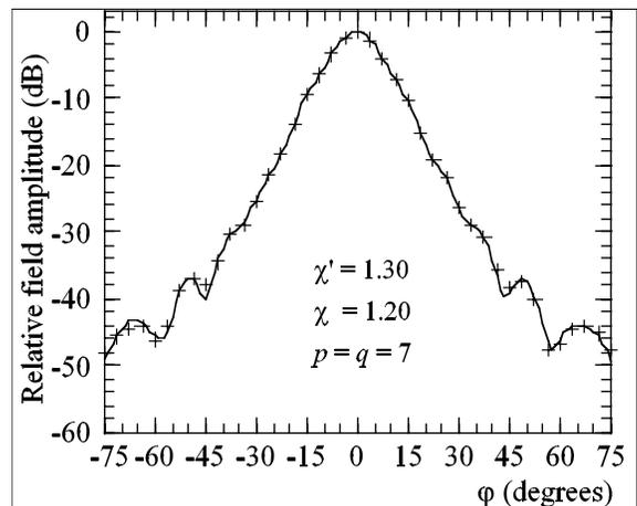
Fig. (7). H-plane pattern. Solid line: reference. Crosses: reconstructed from NF data acquired *via* helicoidal scanning.
