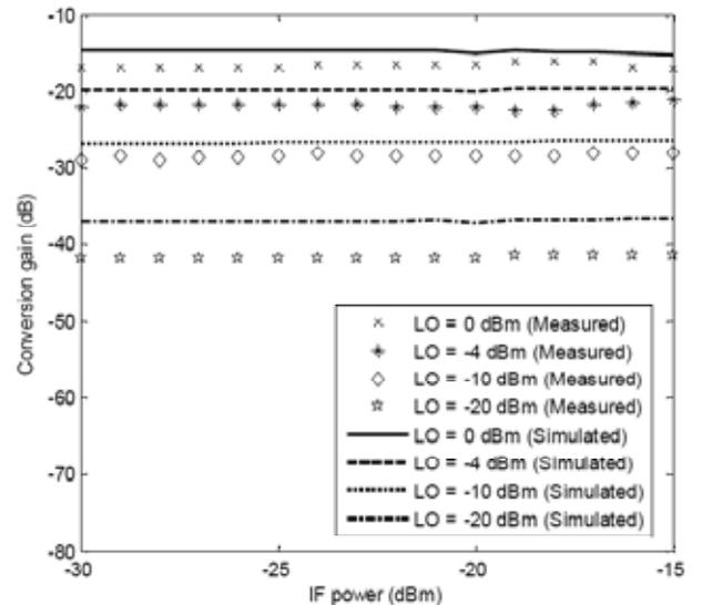
**Fig. (10).** Comparison of measured and simulated of system up-conversion gain versus IF optical modulated power level as a function of LO power.
