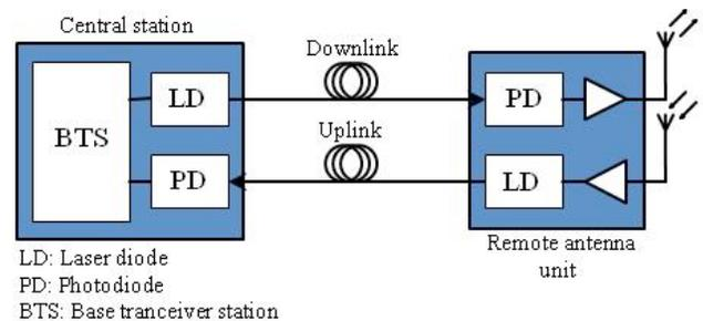
**Fig. (1).** Block diagram of RoF system.
