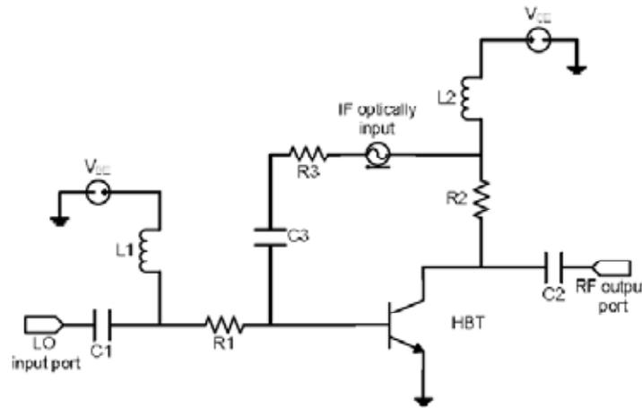
Fig. (2). HBT up-converter circuit mixer for harmonic balance simulation.
