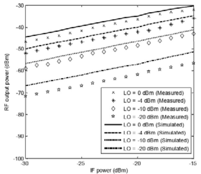
**Fig. (9).** Comparison of measured and simulated of RF output power versus IF optical modulated power level as a function of LO power.
