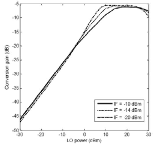
Fig. (6). System conversion gain as a function of LO input power,  $V_{BE} = 0.74$  V and  $V_{CE} = 15$  V.
