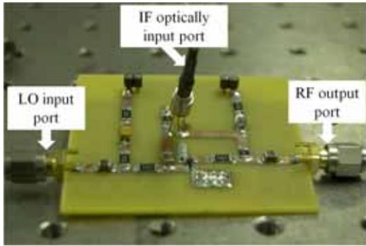
Fig. (4). HBT mixer board circuit for up-conversion 400 MHz to 3.4 GHz.
