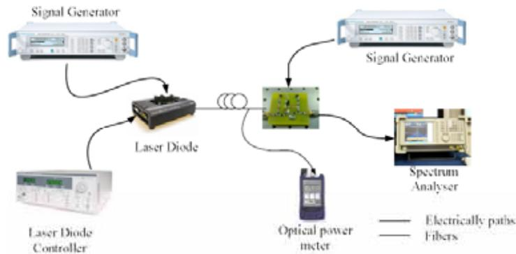
Fig. (3). Experimental arrangement of the 3.4 GHz optical front-end receiver using RoF setup.
