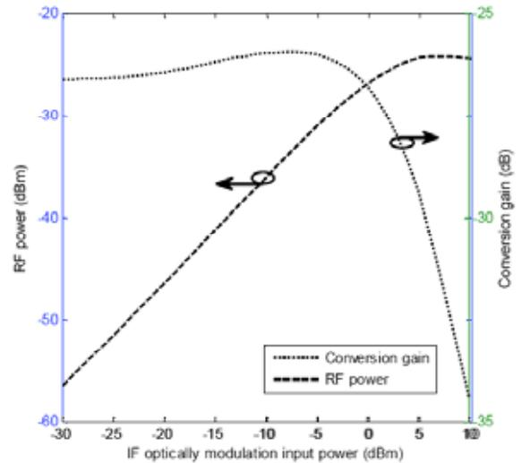
Fig. (7). The conversion gain and RF output power of the BFP640 simulated mixer as a function of IF optical modulated input power at  $V_{BE} = 0.74$  V,  $V_{CE} = 15$  V, and  $P_{LO} = -10$  dBm.
