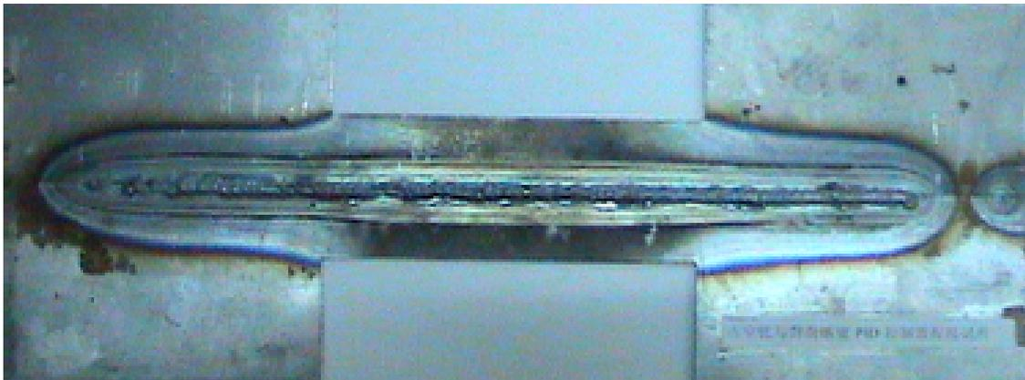
Fig. (4). Weld workpiece of welding speed to backside width of weld Pool with PID controller under the condition of varied heat sink.
