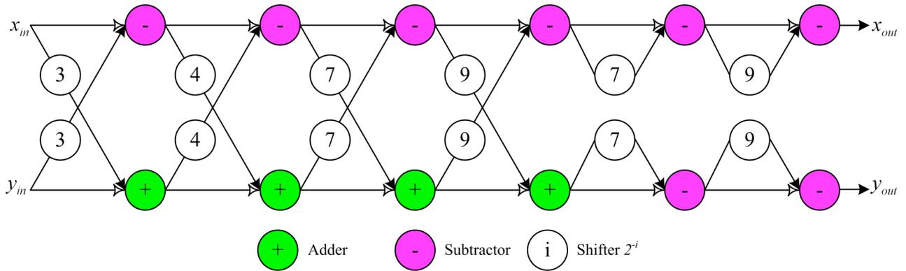
Fig. (6). Unfolded CORDIC flow graph of the  $-\pi/16$ .
