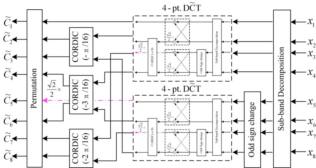
Fig. (3). Signal flow graph of the 8-point DCT.
