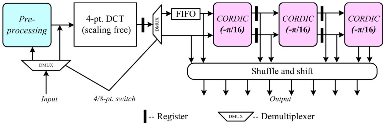
Fig. (9). The reconfigurable 4/8-point DCT architecture based on the modified unfolded CORDIC.
