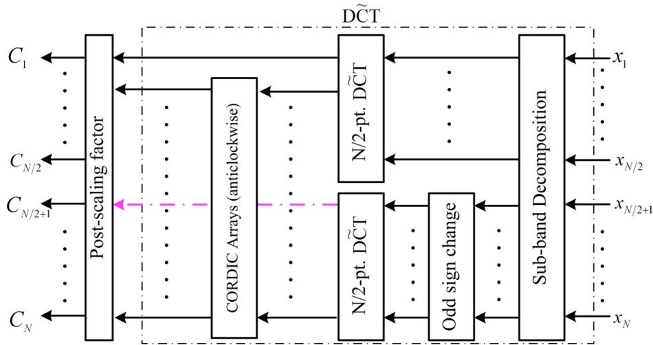
Fig. (4). Signal flow graph of the N-point DCT.
