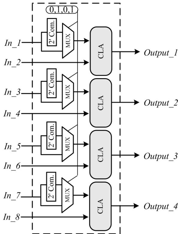
Fig. (10). The architecture of the pre-processing element.
