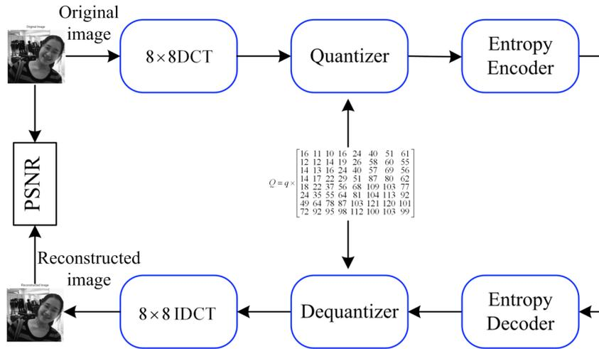
Fig. (11). Block diagram of DCT based JPEG process.
