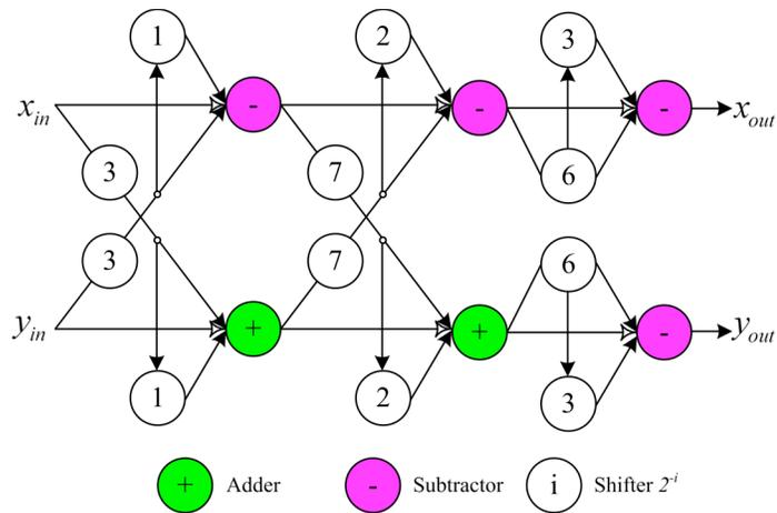
Fig. (7). Modified unfolded CORDIC flow graph of the  $-\pi/16$ .
