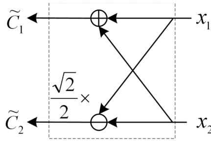
Fig. (1). Signal flow graph of the 2-point DCT.
