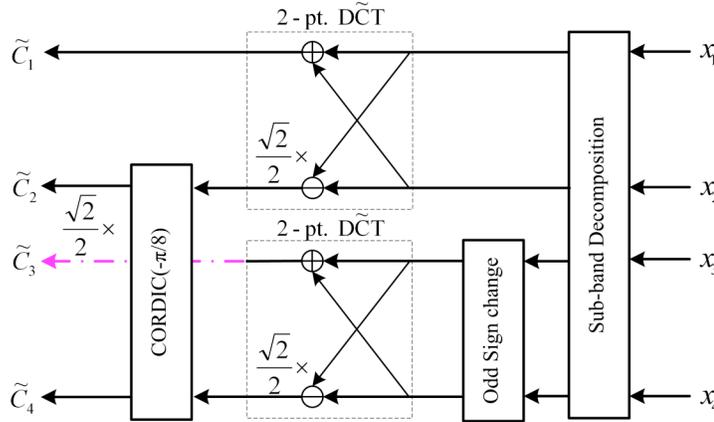
Fig. (2). Signal flow graph of the 4-point DCT.
