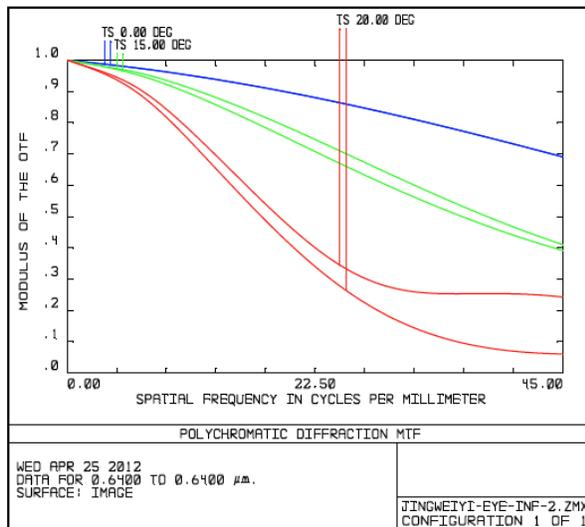
Fig. (6). MTF curves of eyepiece.
