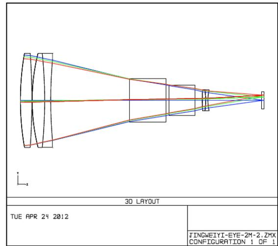
Fig. (3). Telescope system objective optical path.
