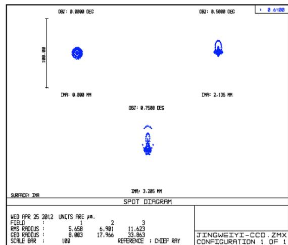
Fig. (8). Spot diagram of CCD receiving system.
