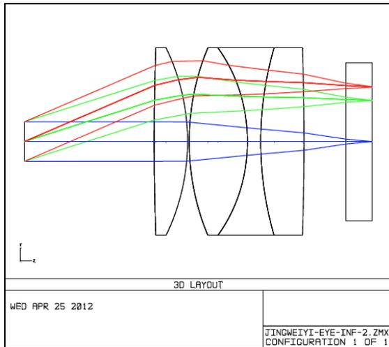
Fig. (5). Optical roadmap of eyepiece.
