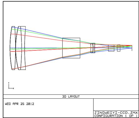
Fig. (7). Optical path of CCD receiving system.
