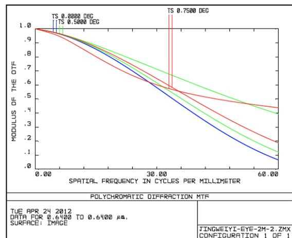
Fig. (4). MTF curves of objective lens.
