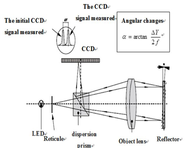
Fig. (1). Principle of photoelectric autocollimator.
