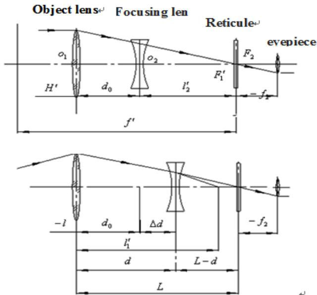
Fig. (2). Diagram of inner focusing system.
