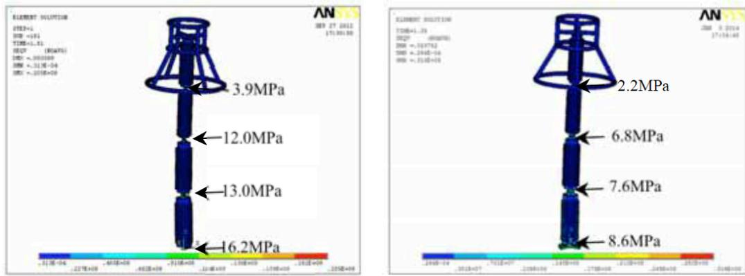
(1) Aseismic structure
