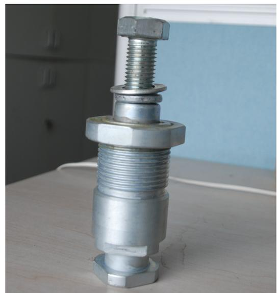
**Fig. (1).** New type lead damper.
