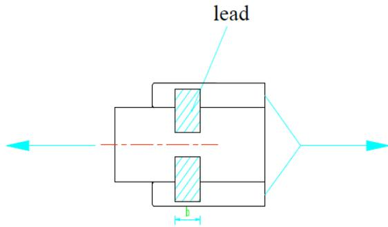
Fig. (2). Action principle of the new type lead damper.
