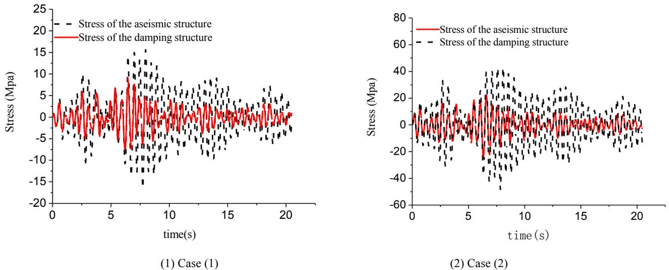
Fig. (6). Stress time history near the root of the UHV porcelain arrester.
