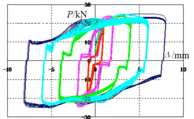
Fig. (3). Hysteretic loops of the new type lead damper.
