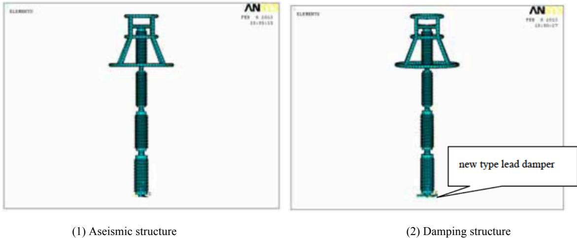
Fig. (5). The finite element models of the UHV porcelain arrester.
