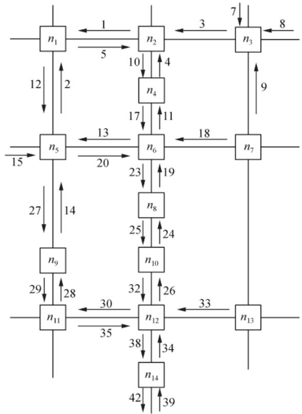
Fig. (3). The topology diagram of the regional road network.
