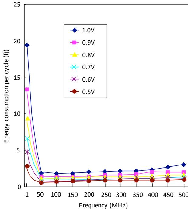
Fig. (10). Energy consumptions per cycle of the FinFET mode-10 counter based on PAL-2N from 1MHz to 500MHz with various source voltages.
