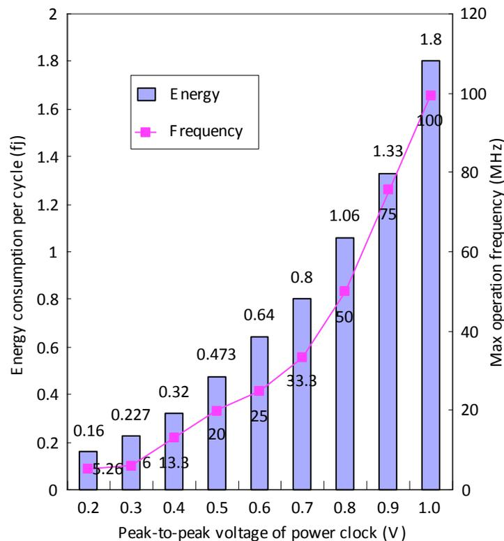
**Fig. (11).** Minimum energy consumption per cycle and corresponding operating frequency of the mode-10 counter based on FinFET from 0.2V to 1.0V.
