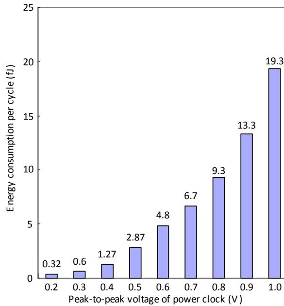
Fig. (7). Energy consumptions of the FinFET mode-10 counter based on PAL-2N from 0.2V to 1.0V at 1 MHz.
