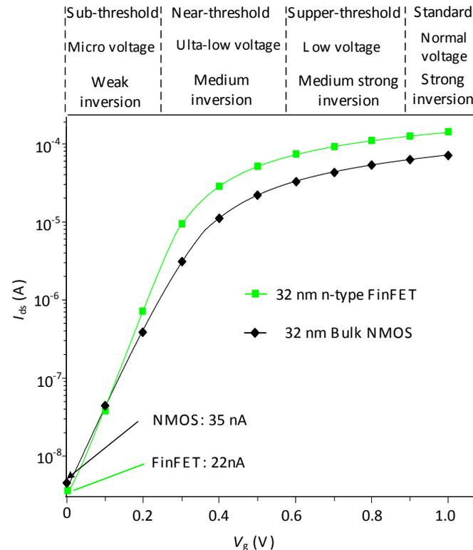
Fig. (2). I -V characteristics of 32 nm n-type FinFET and NMOS bulk transistors.
