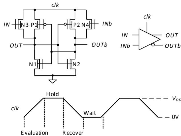
Fig. (4). FinFET buffer/inverter based on PAL-2N: schematic, symbol, and power clock.
