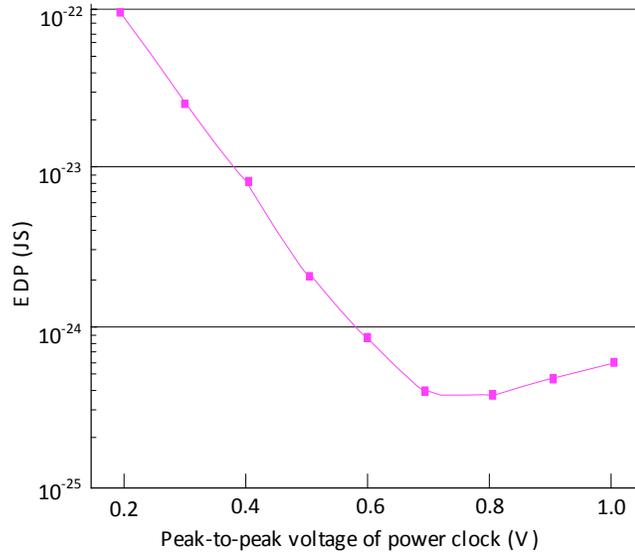
Fig. (9). EDP of the FinFET mode-10 counter based on PAL-2N from 0.2V to 1.0V supply voltages.
