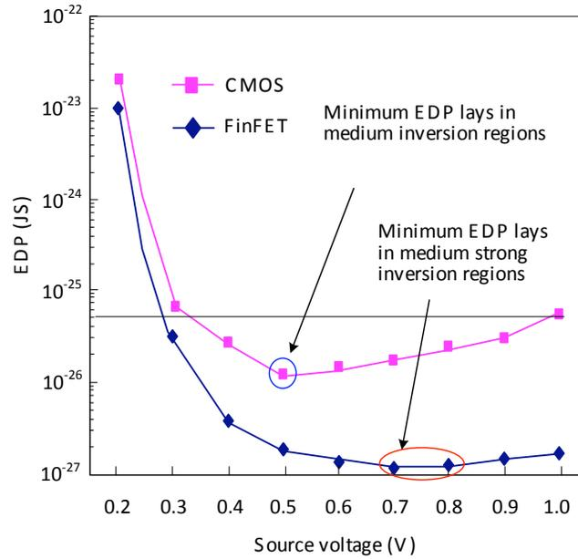
Fig. (3). EDP comparisons of 32nm FinFET and conventional bulk CMOS inverters.
