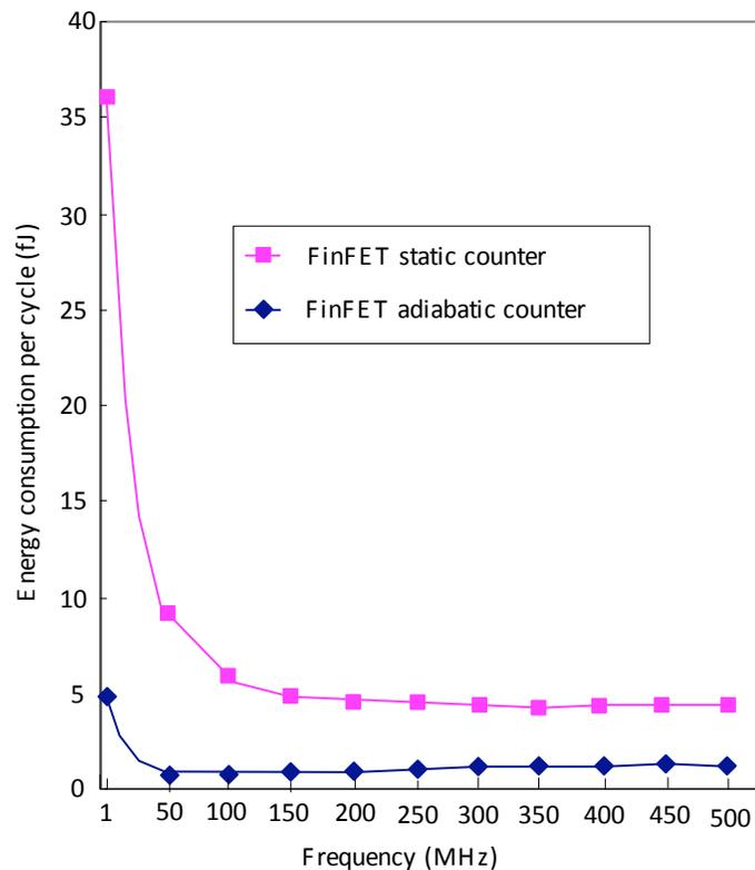
Fig. (12). Energy dissipation comparisons between FinFET adiabatic and conventional mode-10 counters at 0.8V supply voltage.
