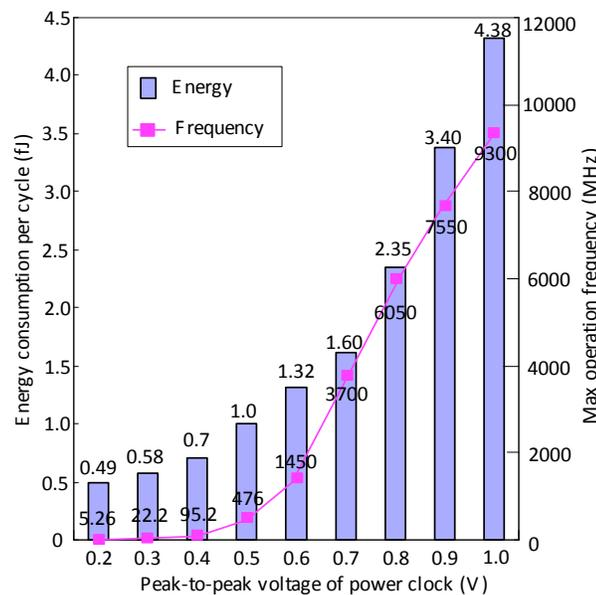
Fig. (8). Max operating frequency and corresponding energy consumptions of the FinFET mode-10 counter based on PAL-2N from 0.2V to 1.0V supply voltages.
