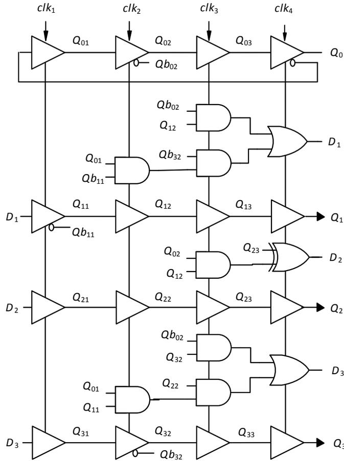
Fig. (6). Adiabatic FinFET mode-10 counter based on PAL-2N circuits.
