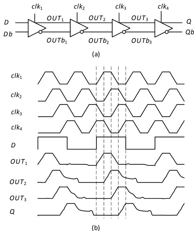
Fig. (5). FinFET PAL-2N flip-flop. (a) D flip-flop, and (b) Simulation waveforms of D flip-flop.
