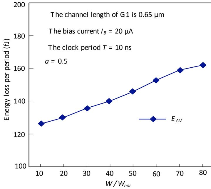
**Fig. (10).** Average energy loss per period of the power-gating circuits *versus* channel width of the power-gating transistor.  $W_{nor}$  is 1.04  $\mu\text{m}$ .
