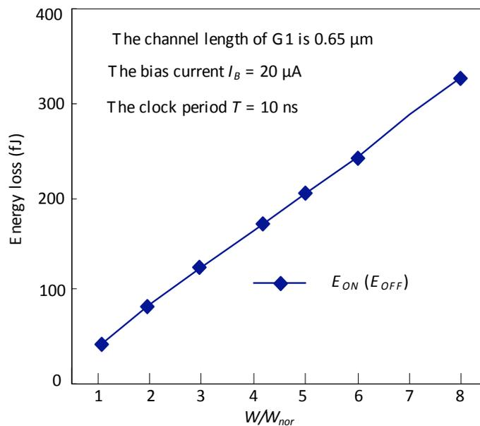
Fig. (9). Energy loss for turning on and off the power-gating switch G1 versus channel width of the power-gating transistor.  $W_{nor}$  is  $1.04 \mu\text{m}$ .
