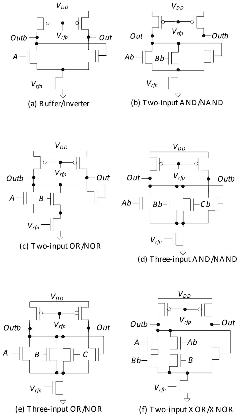
Fig. (2). Basic SRMCMCML gates.
