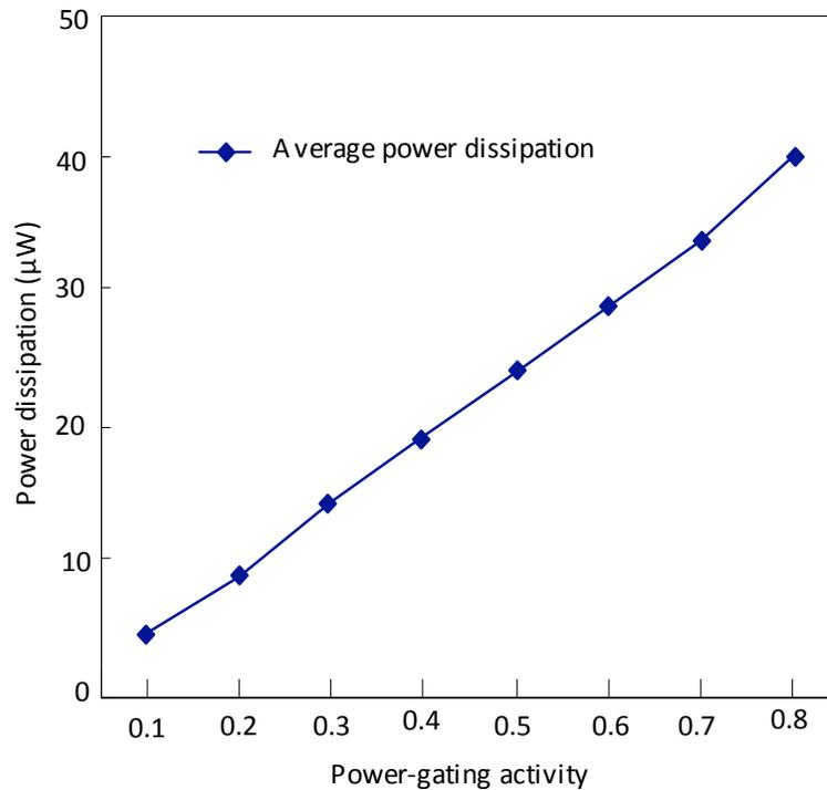
Fig. (14). Power dissipations of the power-gating SRMCML full adder with various power-gating active ratios.
