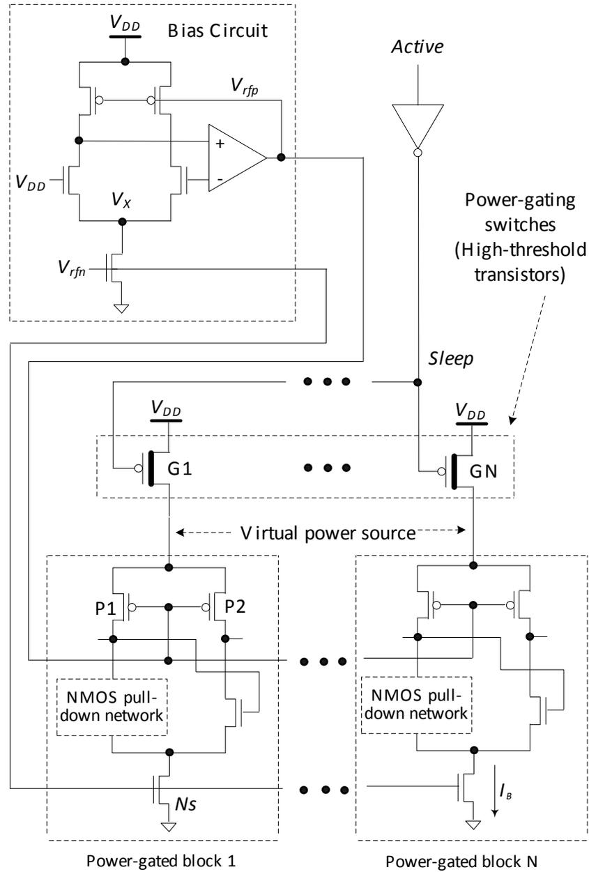
Fig. (3). Power-gating scheme for SRMCML circuits.
