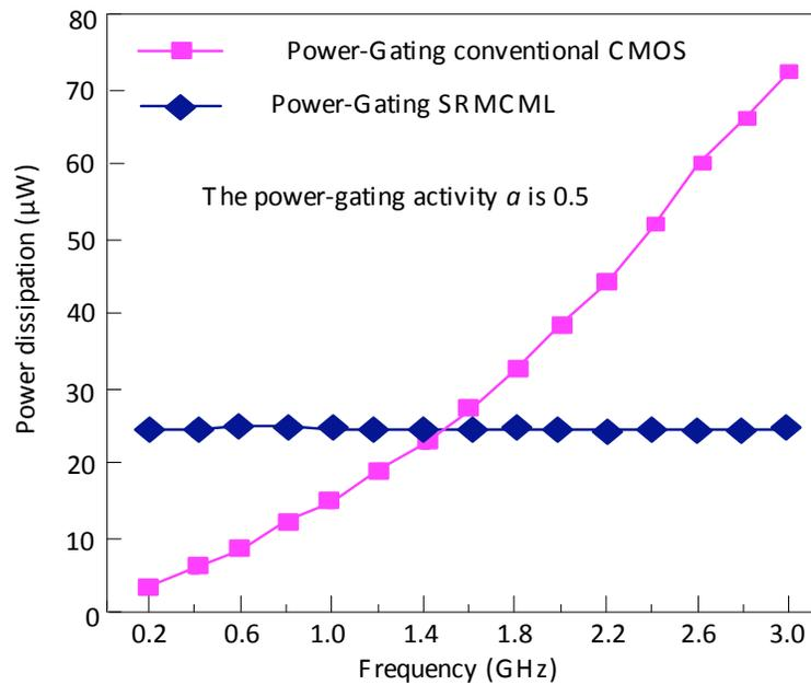
Fig. (13). Power consumption comparison between the power-gating SRMCML and conventional CMOS full adders.
