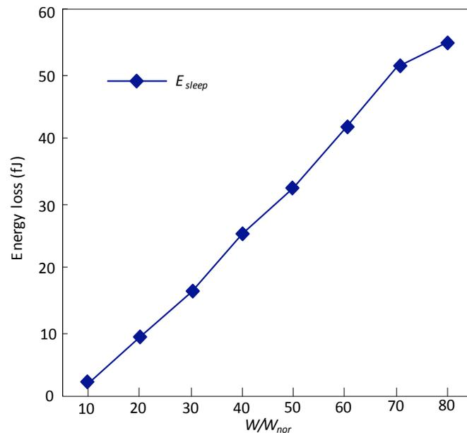
Fig. (8). Energy loss versus channel width of the power-gating switch G1 in sleep mode.  $W_{nor}$  is  $1.04 \mu\text{m}$
