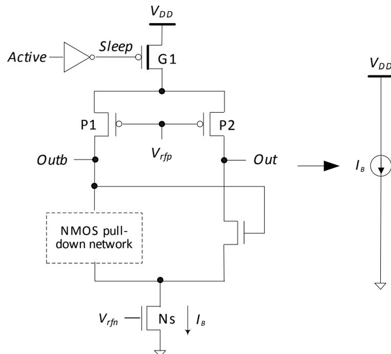
Fig. (5). Equivalent circuit for calculating the energy dissipation of the power-gating circuits in active mode.
