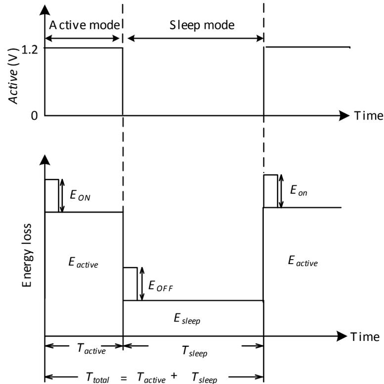
Fig. (4). Operation schedule and energy loss of power-gating SRMCMCML circuits.
