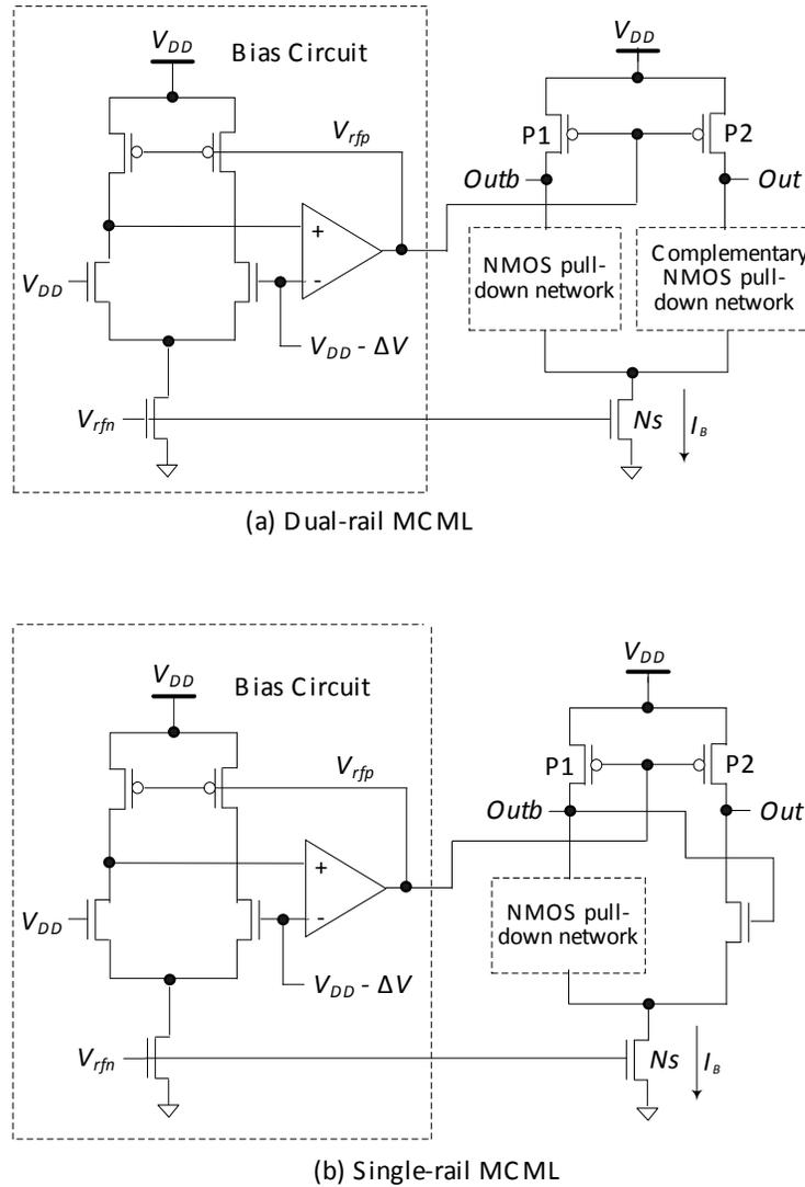
Fig. (1). MCML circuits with dual-rail and signal schemes.
