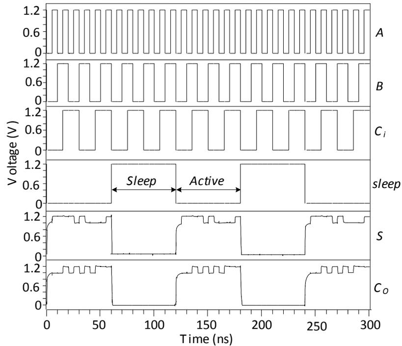
Fig. (12). Simulation waveforms of the power-gating 1-bit full adder based on SRMCML.
