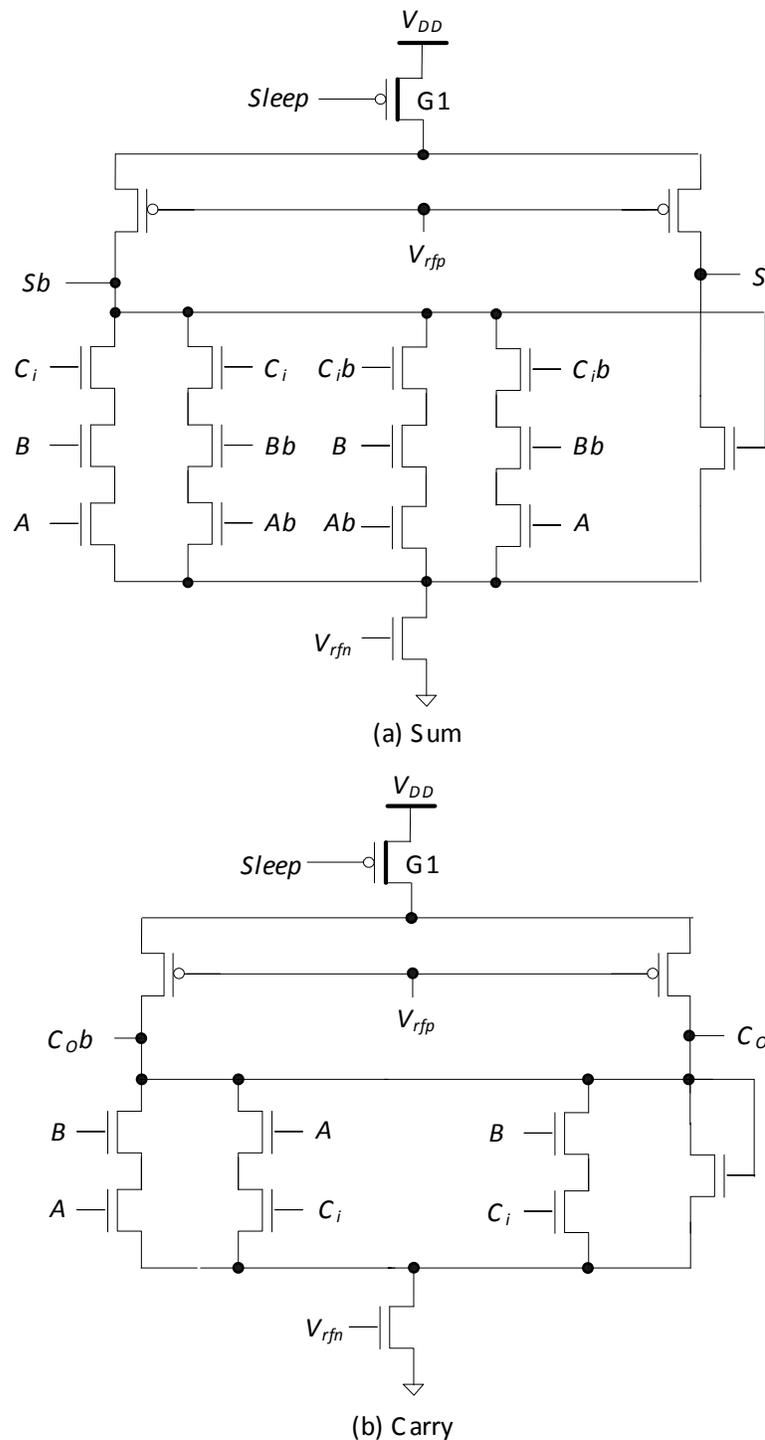
Fig. (11). Power-gating 1-bit full adder based on SRMCMCML.
