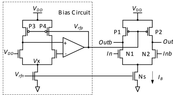
Fig. (1). MCML inverter/buffer and its bias circuit.
