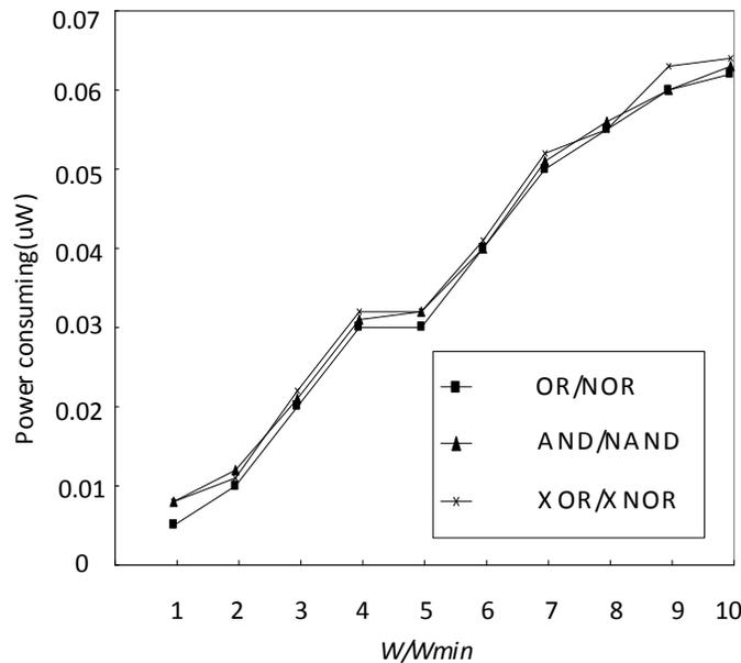
Fig. (9). Power consuming of the proposed power-gating MCML basic gates in sleep mode versus channel width of power-gating switches at 800MHz ( $W_{min}=0.52\mu m, L=0.65\mu m$ ).
