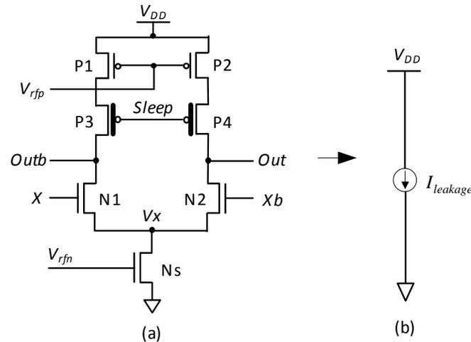
Fig. (8). Equivalent model when circuit works in sleep mode.
