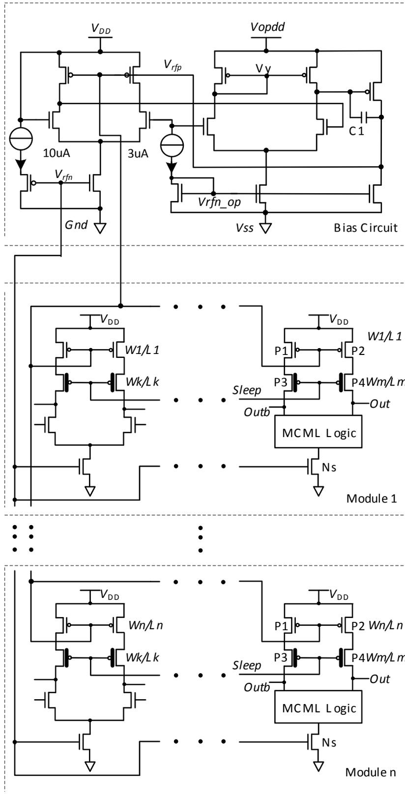
Fig. (3). The proposed power-gating MCML circuits where the widths and lengths of sleep transistors in power-gated blocks are separately adjusted.
