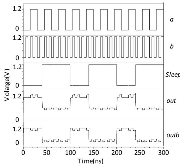
Fig. (5). Simulation waveforms of the proposed power-gating MCML AND2/NAND2.
