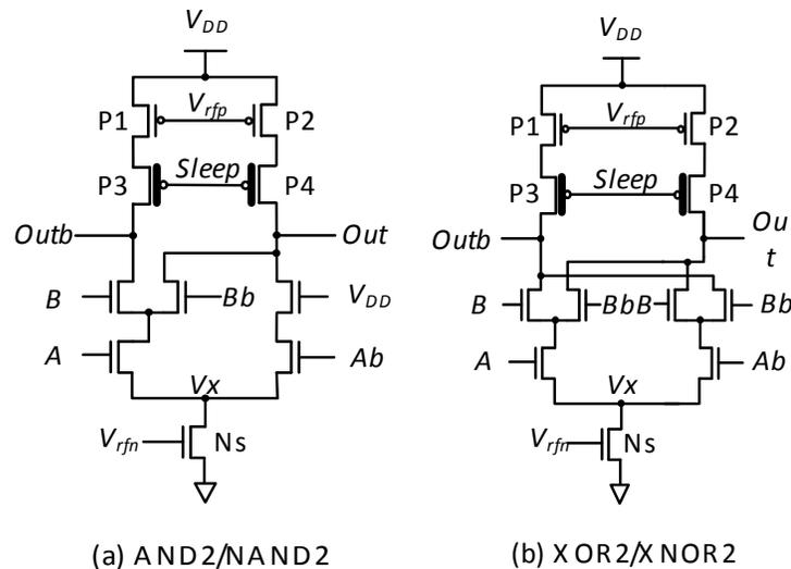
Fig. (4). Basic gates based on the proposed power-gating scheme.
