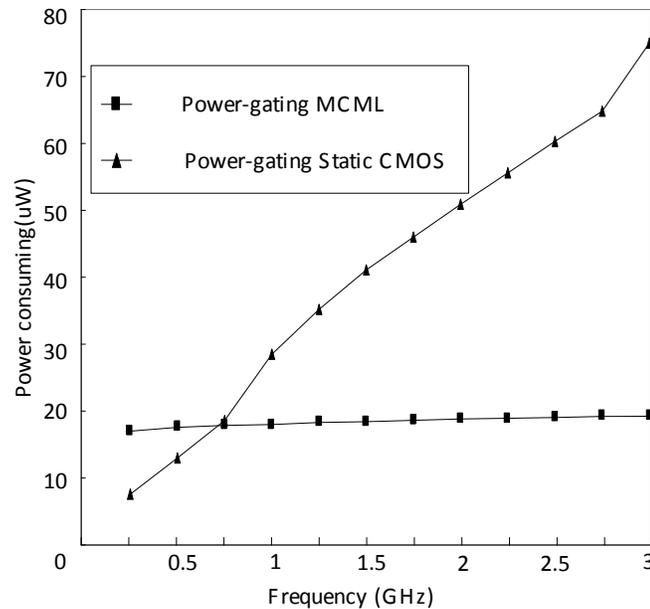
**Fig. (12).** Power dissipation of power-gating static CMOS logic and power-gating MCML 1 bit full adders (active ratio=0.6) with various frequencies.
