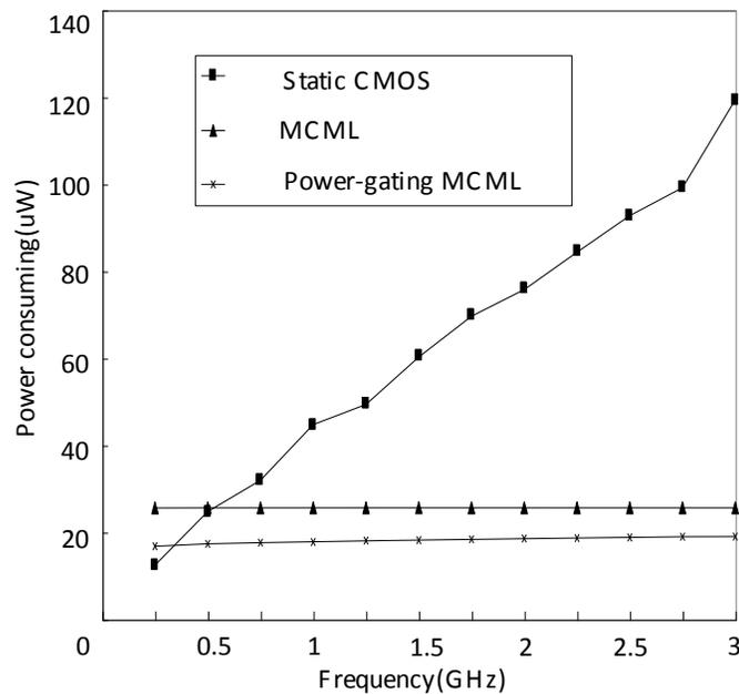
Fig. (11). Power dissipation of static CMOS logic, MCML and power-gating MCML 1 bit full adders (active ratio=0.6) with various frequencies.
