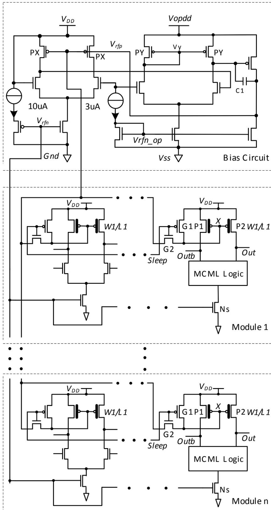
**Fig. (2).** Power-gating MCML circuits whwer the widths and lengths of sleep transistors in power-gated blocks are dependent on the bias circuit.
