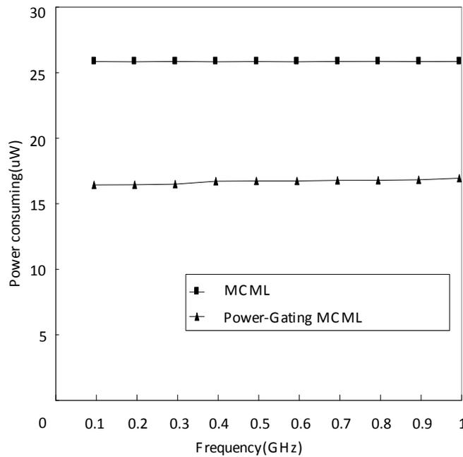
Fig. (10). Power consumption of conventional MCML 1 bit full adder and the power-gating 1-bit full adder that based on the proposed scheme with an active ratio of 0.6.
