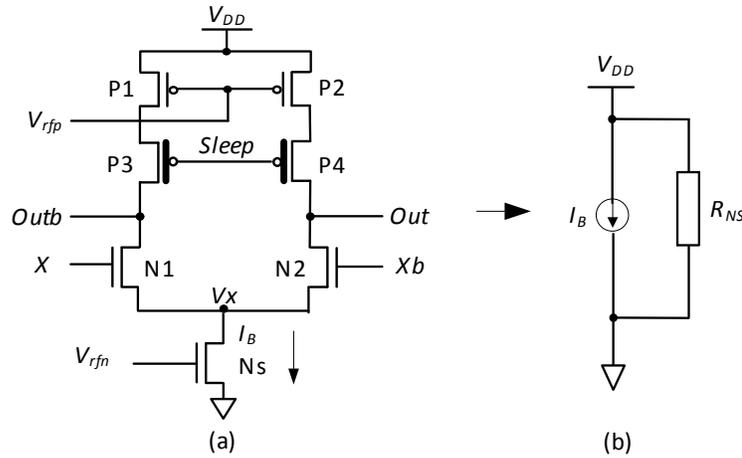
Fig. (6). Equivalent model when circuit works in active mode.
