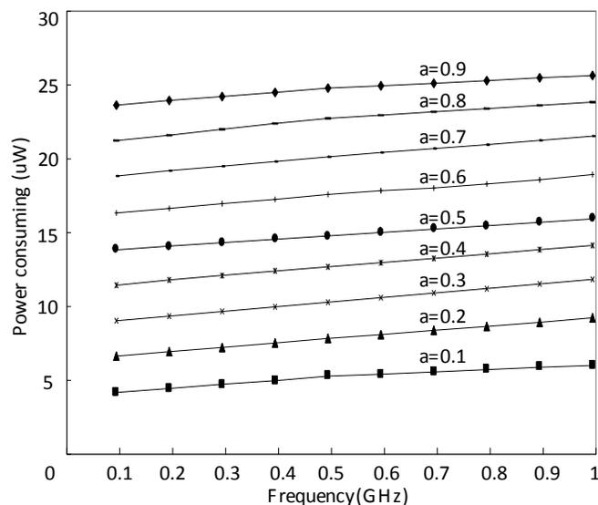
**Fig. (13).** Power consuming of proposed power-gating MCML 1 bit full adder with various active ratios.
