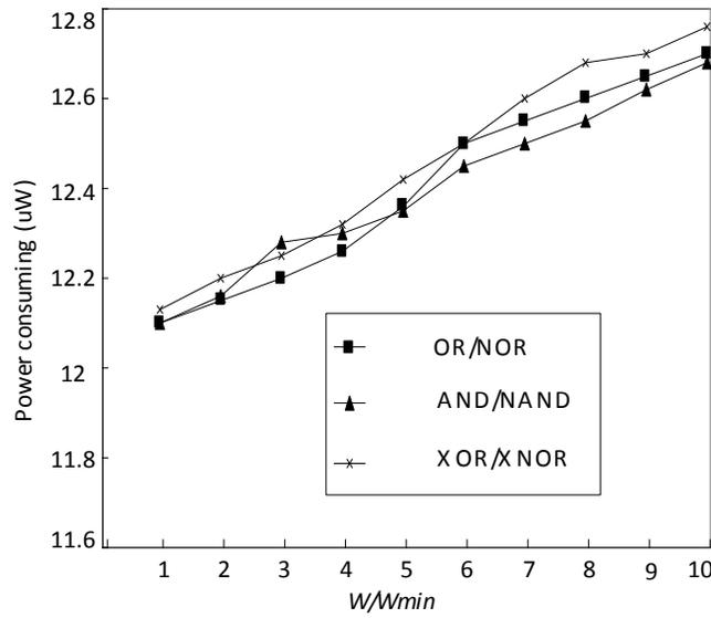
Fig. (7). Power consuming of the proposed power-gating MCML gates in active mode versus channel width of power-gating switches at 800MHz ( $W_{min} = 0.52\mu\text{m}$ ,  $L = 0.65\mu\text{m}$ ).
