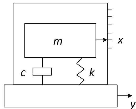
**Fig. (1).** Mechanical model of piezoelectric type acceleration sensor.
