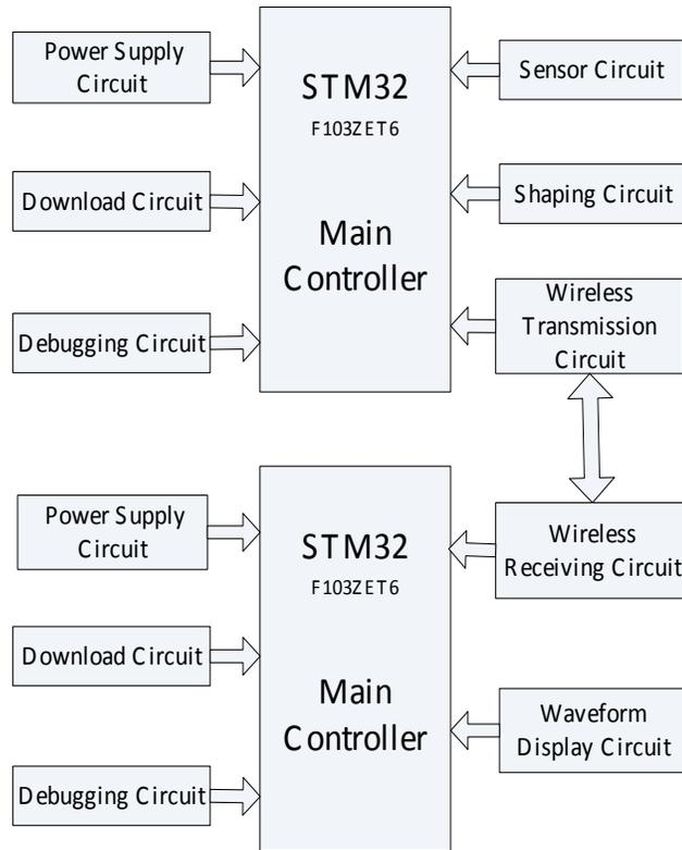
Fig. (2). Hardware design block diagram of the system.
