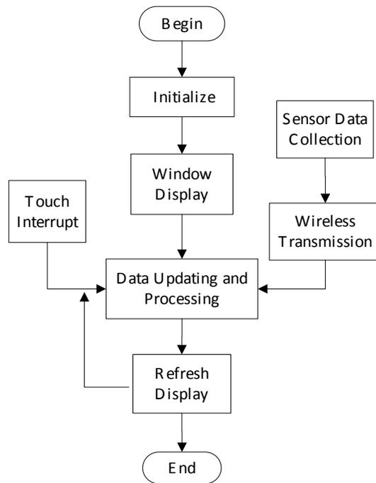
Fig. (4). Flow diagram of the main program.
