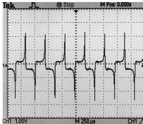
(a) Carrier signal waveform
