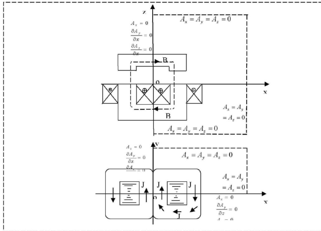
Fig. (1). The determination of boundary condition on U electromagnet.
