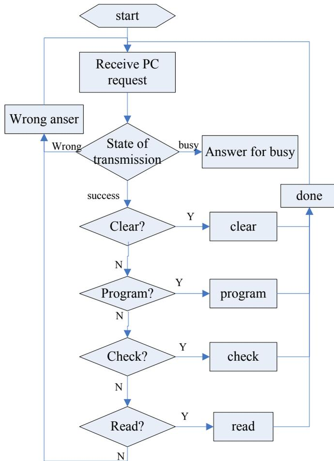
Fig. (8). The program flow chart of the lower computer.
