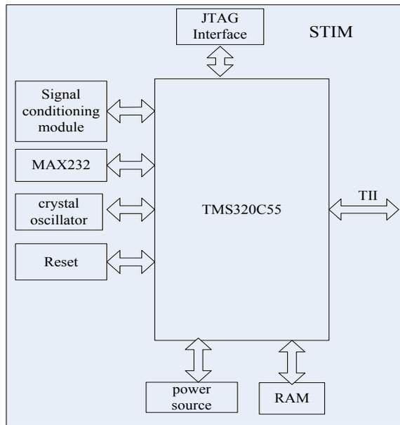
Fig. (6). STIM principle block diagram.
