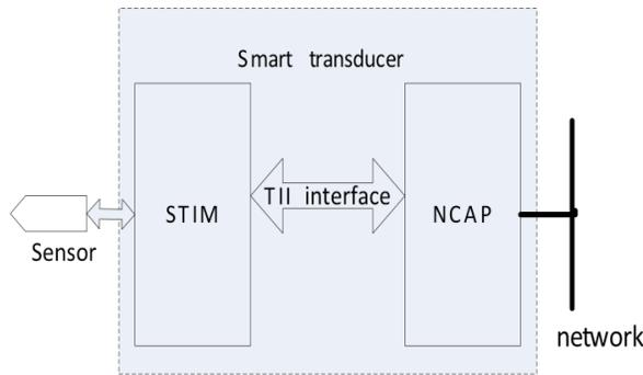
Fig. (2). Smart transducer structure.
