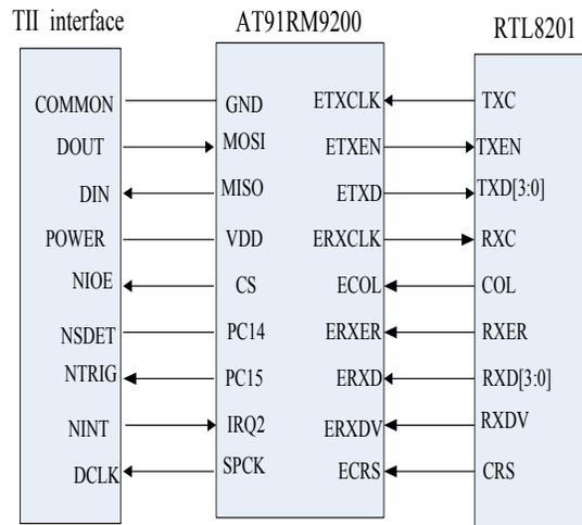
Fig. (4). The connection between microprocessor and network signal processor.
