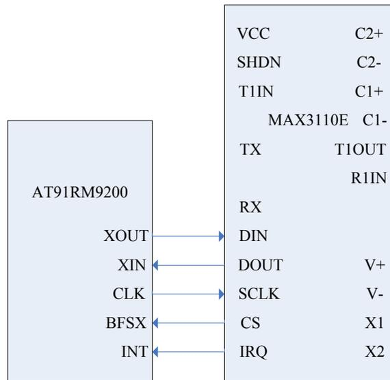
Fig. (5). The connection between AT91RM922 and MAX3110E.
