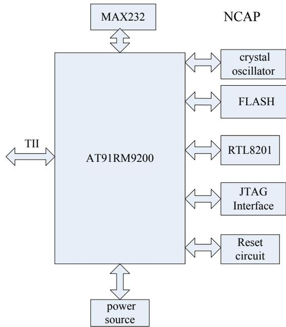
Fig. (3). NCAP principle block diagram.
