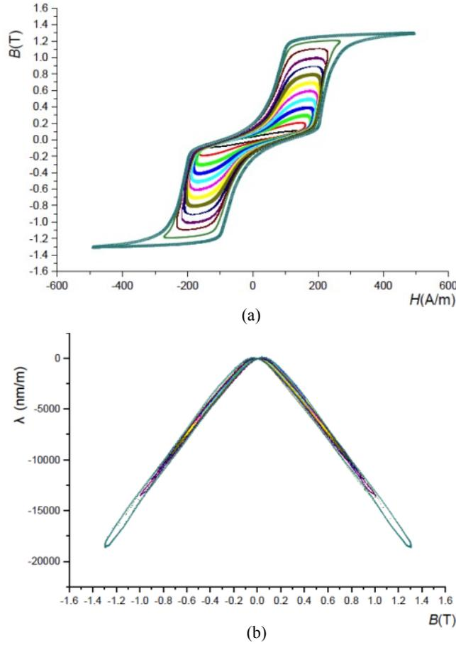
**Fig. (1).** AC magnetic characteristics curves of one type grain oriented steel in RD with 50Hz. (a) Hysteresis loops. (b) Magnetostriction butterfly curves
