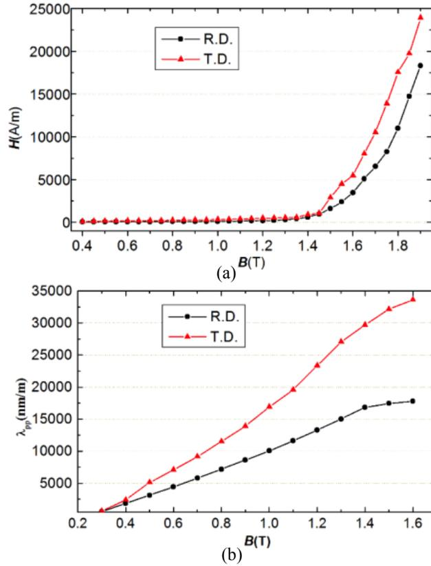
**Fig. (2).** The magnetization curves and peak-to-peak MS values in RD and TD of the type grain oriented steel. (a) Magnetization curves. (b) Peak-to-peak MS values.
