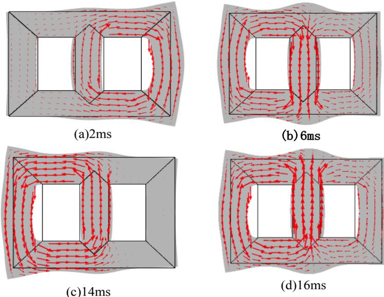
Fig. (4). Section view of magnetic flux and deformation distribution of the transformer core.
