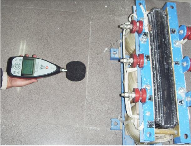
Fig. (6). Sound pressure level measurement.
