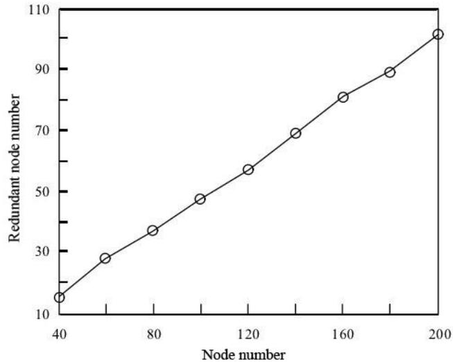
Fig. (2). The number of redundant nodes in wireless sensor network with different nodes.
