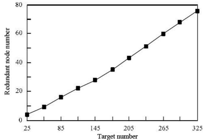
Fig. (3). The number of redundant targets for different targets in wireless sensor network.
