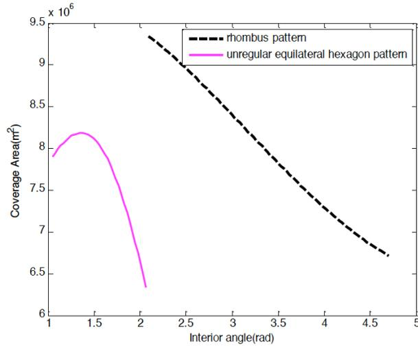
Fig. (7). The coverage area when using 3600 combination round deployed in rhombus and irregular equilateral hexagon pattern.
