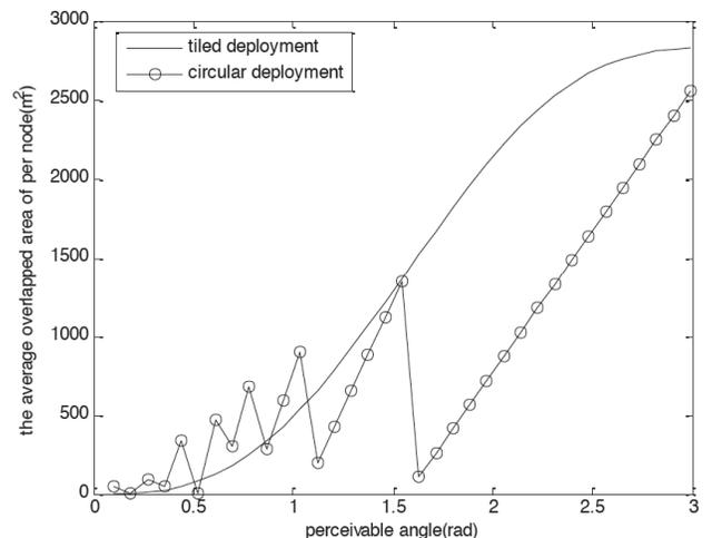
Fig. (3). The comparison between circular deployment and tiled deployment.
