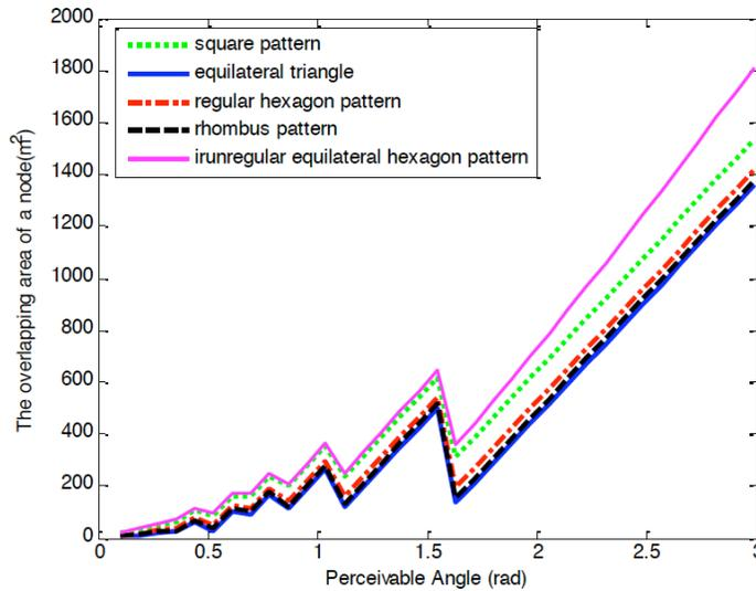
Fig. (9). The overlapping area of a node of different specification graphical deployment.
