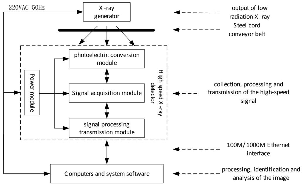
Fig. (1). The structure frame of steel cord conveyor belt detection system.
