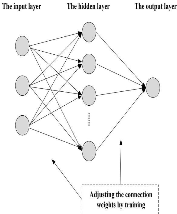
Fig. (1). Neural network structure diagram.
