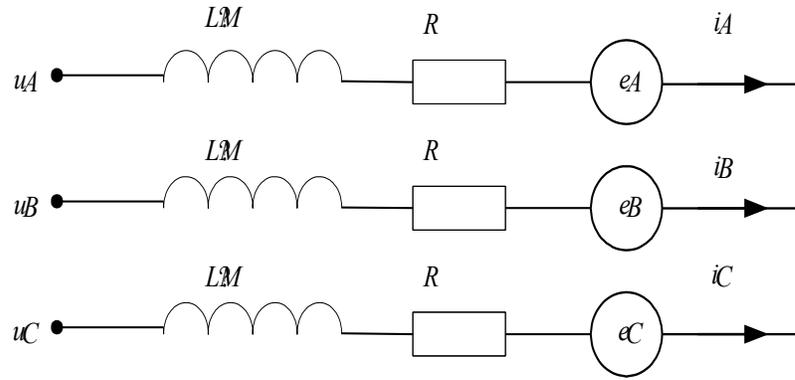
Fig. (1). Equivalent circuit of brushless DC motors.
