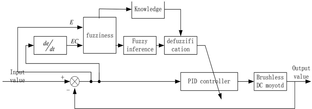
Fig. (2). Conceptual design of fuzzy rotation rate PID control.
