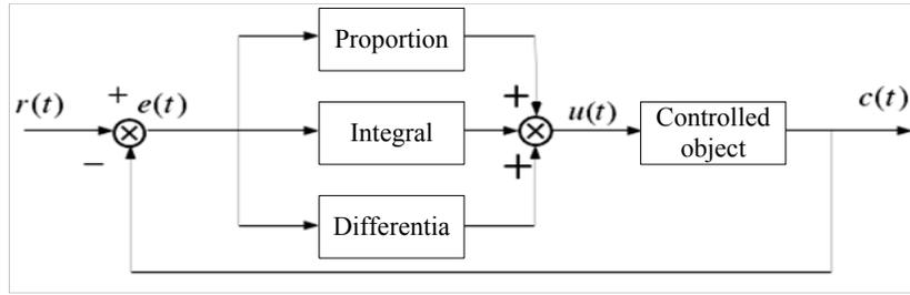
Fig. (3). The principle of the PID control.
