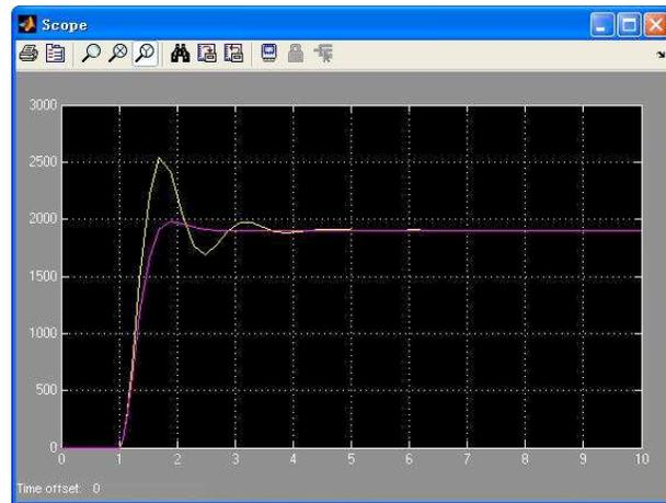
Fig. (8). Output comparison of pure proportion factor control and proportion-differential control PID system.
