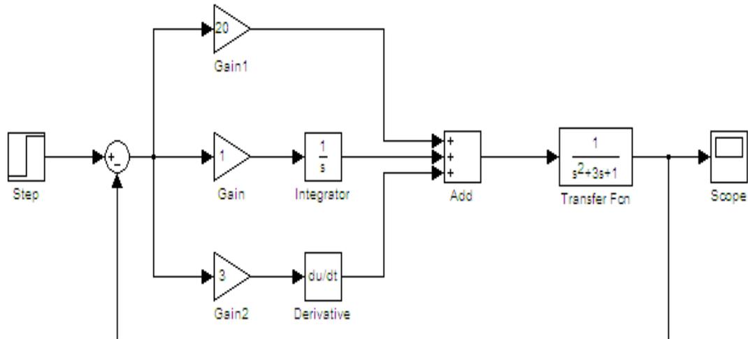
Fig. (6). PID control system modeling under SIMULINK.
