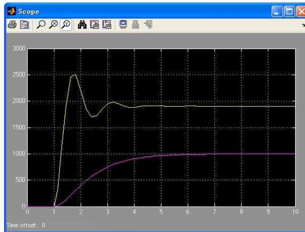
Fig. (7). Influence of proportion factor  $k_p$  on the PID system under pure proportional control.
