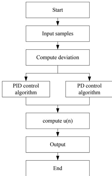
Fig. (4). Integral separated control algorithm flowchart.
