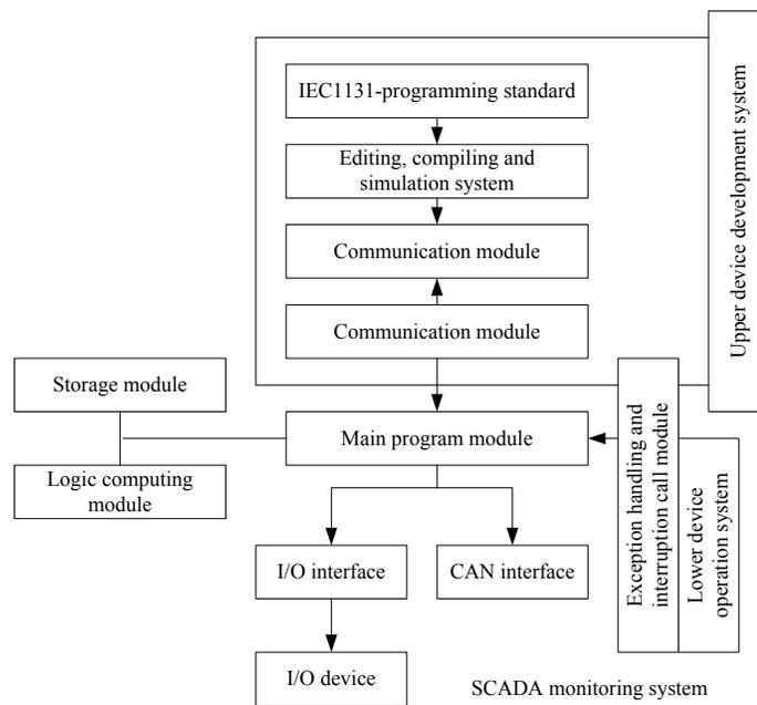
Fig. (2). Soft PLC software system structure.
