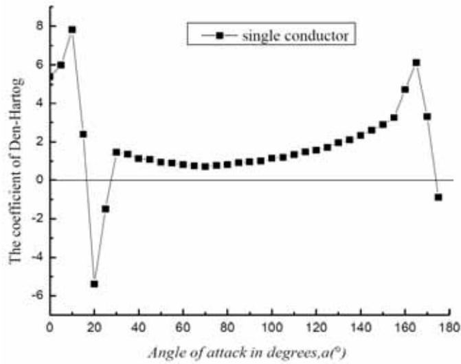
**Fig. (8).** The coefficient of Den-Hartog of iced single conductor.
