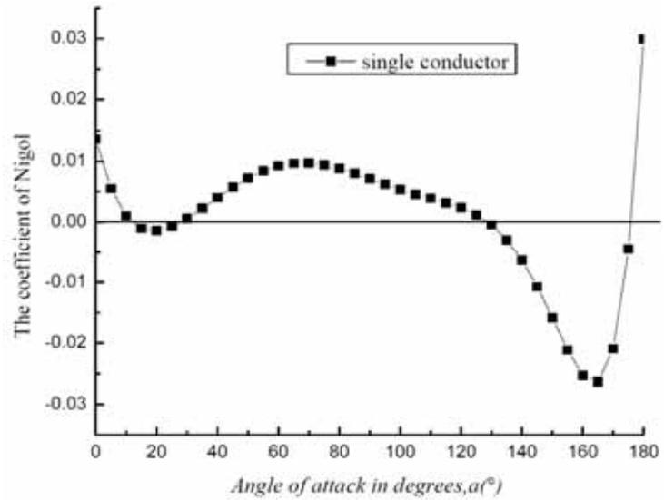
**Fig. (9).** The coefficient of Nigol of iced single conductor.
