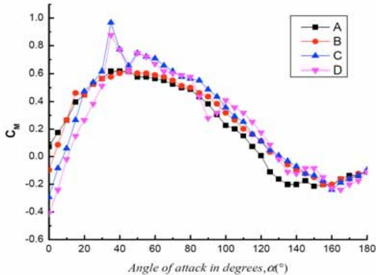
Fig. (5). Moment coefficient of iced four bundled conductors.
