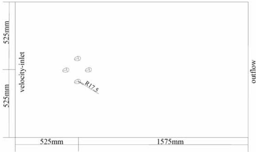
Fig. (1). Schematic diagram of rectangular area.
