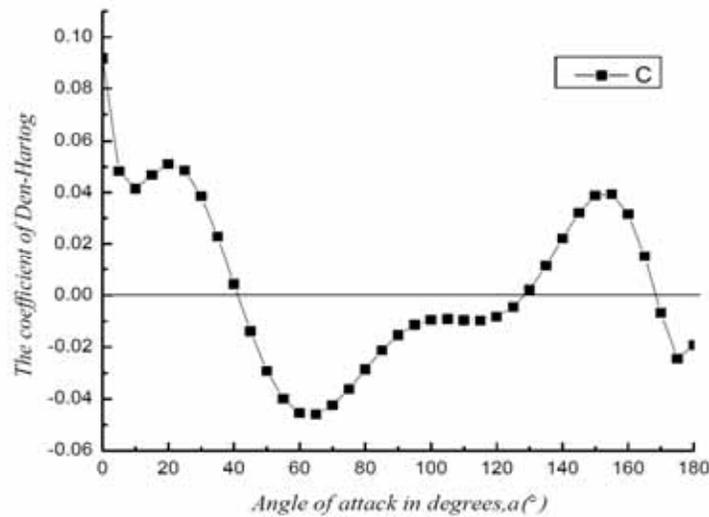
Fig. (6). The Den-Hartog coefficient of C.
