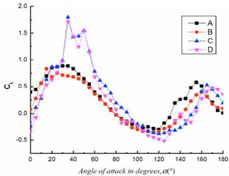
Fig. (3).Lift coefficient of iced four bundled conductors.
