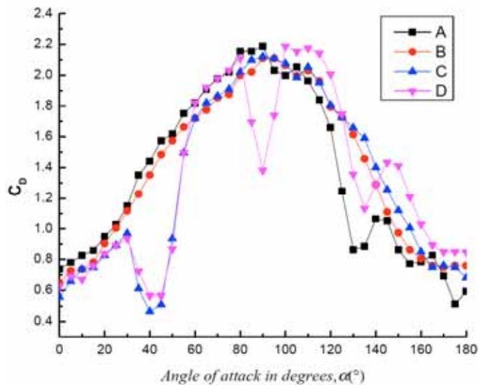
Fig. (4). Drag coefficient of iced four bundled conductors.
