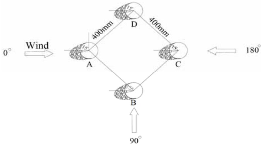
Fig. (2). The modal of four bundled conductors with crescent section.
